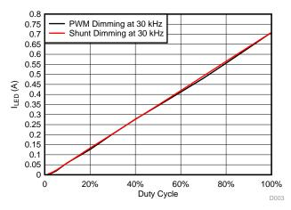
Figure 29. I<sub>LED</sub> (A) versus Duty Cycle (%) for PWM or Shunt Dimming at 30 kHz for Blue LED String
