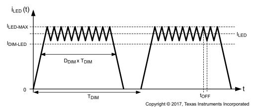
Figure 15. LED Current I<sub>LED</sub>(t) During EN Pin PWM Dimming
