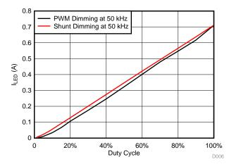
Figure 32. I<sub>LED</sub> (A) versus Duty Cycle (%) for PWM or Shunt Dimming at 50 kHz for Green LED String
