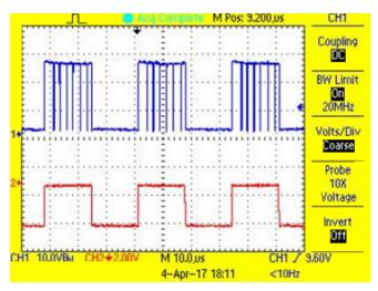
Figure 53. Switch Node and Shunt PWM Waveform for White LED String at 50% Duty Cycle
