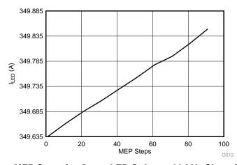
Figure 18. I<sub>LED</sub> versus MEP Steps for Green LED String at 30-kHz Shunt Dimming Frequency
