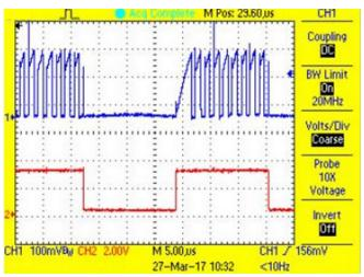
Figure 40. P-FET Current During On-Time and PWM
