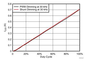
Figure 28. I<sub>LED</sub> (A) versus Duty Cycle (%) for PWM or Shunt Dimming at 30 kHz for Green LED String
