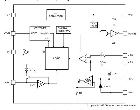
Figure 5. Functional Block Diagram of LM3409
