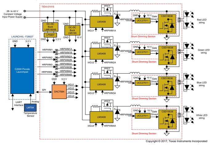
Figure 4. TIDA-01415 Block Diagram
