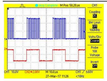
Figure 51. Switch Node and Shunt PWM Waveform for Blue LED String at 50% Duty Cycle
