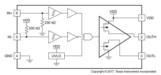
Figure 7. Functional Block Diagram of UCC27511
