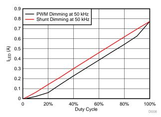
Figure 34. I<sub>LED</sub> (A) versus Duty Cycle (%) for PWM or Shunt Dimming at 50 kHz for White LED String
