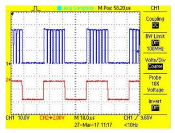
Figure 49. Switch Node and Shunt PWM Waveform for Green LED String at 50% Duty Cycle
