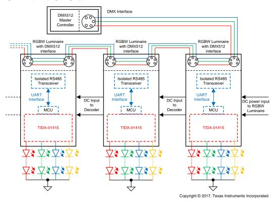
Figure 1. TIDA-01415 End Application in Stage Lighting
