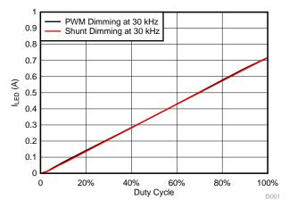
Figure 27. I<sub>LED</sub> (A) versus Duty Cycle (%) for PWM or Shunt Dimming at 30 kHz for Red LED String
