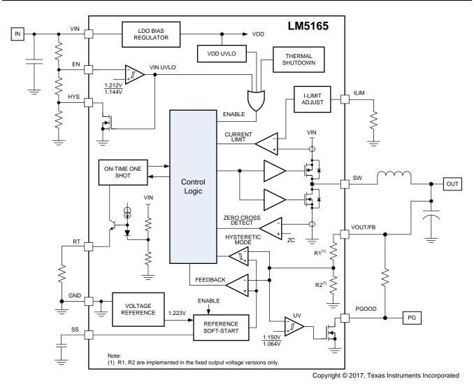
Figure 10. Functional Block Diagram of LM5165
