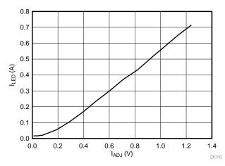
Figure 23. I<sub>LED</sub> (A) versus I<sub>ADJ</sub> (V) for Red LED String
