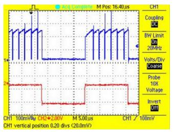
Figure 54. P-FET Current During On-Time and Shunt PWM Waveform for White LED String at 50% Duty Cycle
