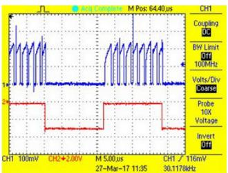
Figure 52. P-FET Current During On-Time and Shunt PWM Waveform for Blue LED String at 50% Duty Cycle
