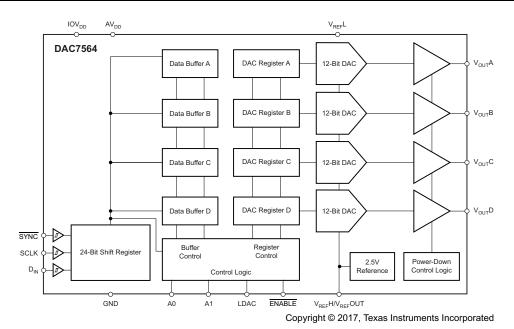
Figure 6. Functional Block Diagram of DAC7564
