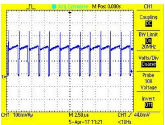
Figure 37. P-FET Current During On-Time at  $I_{ADJ} = 1.24 \text{ V}$  for Blue String
