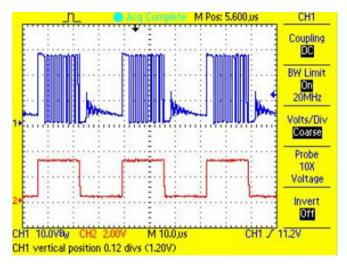
Figure 39. Switch Node and PWM Waveform for Red LED String at 50% Duty Cycle
