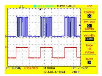
Figure 47. Switch Node and Shunt PWM Waveform for Red LED String at 50% Duty Cycle
