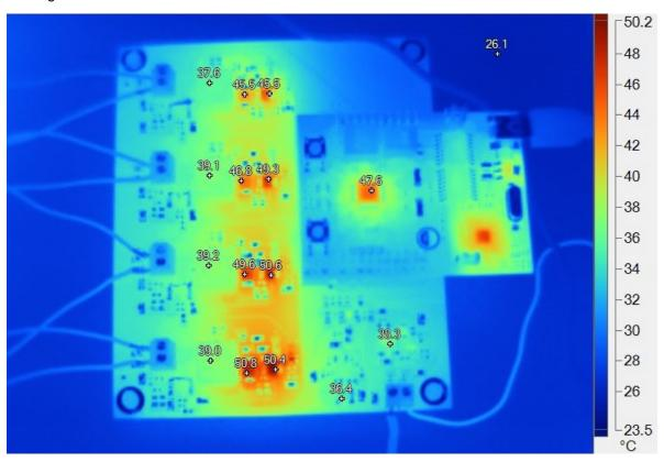
Figure 59. Thermal Image of Top Side of TIDA-01415 Board for PWM Dimming at 2.9-A Total LED Current (100% Duty Cycle for All Strings)
