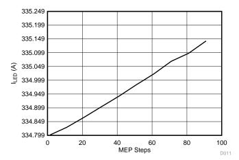
Figure 17. I<sub>LED</sub> versus MEP Steps for Green LED String at 30-kHz PWM Dimming Frequency
