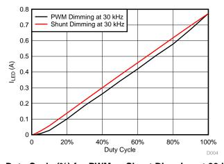
Figure 30. I<sub>LED</sub> (A) versus Duty Cycle (%) for PWM or Shunt Dimming at 30 kHz for White LED String
