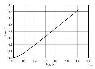
Figure 26.  $I_{LED}$  (A) versus  $I_{ADJ}$  (V) for White LED String
