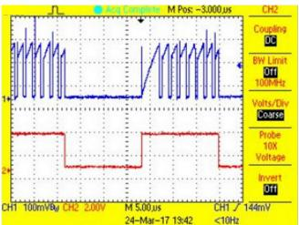
Figure 44. P-FET Current During On-Time and PWM
