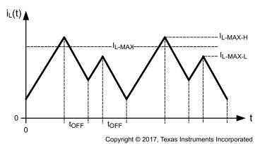
Figure 13. Inductor Current i<sub>L</sub>(t) Showing I<sub>L-MAX</sub> Offset
