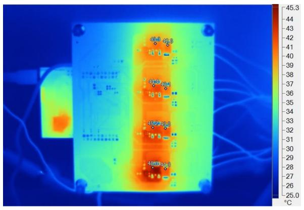
Figure 60. Thermal Image of Bottom Side of TIDA-01415 Board for PWM Dimming at 2.9-A Total LED Current (100% Duty Cycle for All Strings)
