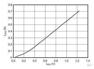
Figure 24. I<sub>LED</sub> (A) versus I<sub>ADJ</sub> (V) for Green LED String
