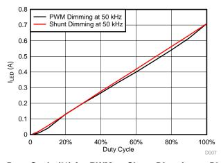
Figure 33. I<sub>LED</sub> (A) versus Duty Cycle (%) for PWM or Shunt Dimming at 50 kHz for Blue LED String
