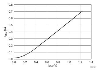
Figure 25.  $I_{LED}$  (A) versus  $I_{ADJ}$  (V) for Blue LED String
