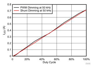
Figure 31. I<sub>LED</sub> (A) versus Duty Cycle (%) for PWM or Shunt Dimming at 50 kHz for Red LED String
