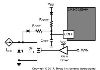
Figure 14. External Parallel FET Dimming Circuit
