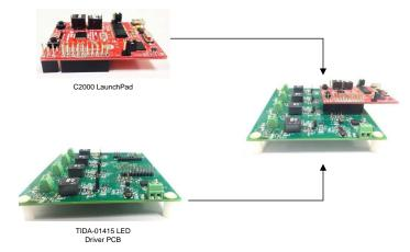
Figure 21. C2000 LaunchPad Mounted on TIDA-01415 LED Driver Board
