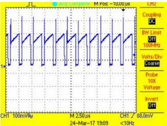
Figure 35. P-FET Current During On-Time at  $I_{ADJ}$  = 1.24 V for Red String
