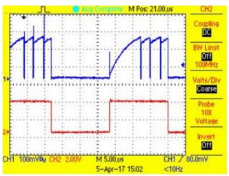
Figure 46. P-FET Current During On-Time and PWM
