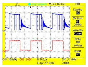
Figure 45. Switch Node and PWM Waveform for White LED String at 50% Duty Cycle
