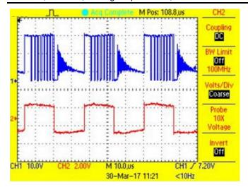
Figure 43. Switch Node and PWM Waveform for Blue LED String at 50% Duty Cycle
