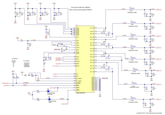
Figure 11. TAS6424-Q1 Class-D Power Audio Amplifier Circuit
