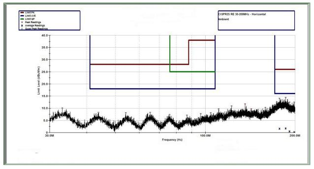
Figure 27. CISPR 25 Radiated Emissions: 30 MHz to 200 MHz, Horizontal Antenna Orientation, Ambient Scan
