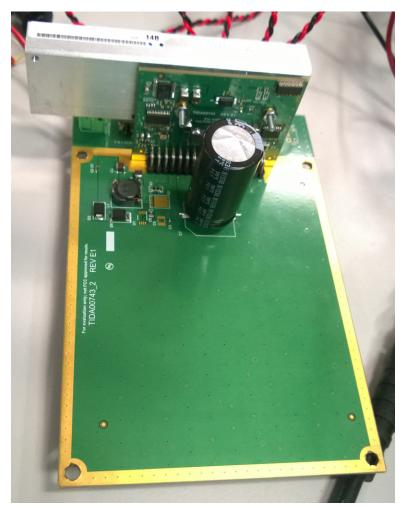
Figure 15. TIDA-00743 Module Board With Heat Sink Attached to Carrier Board
