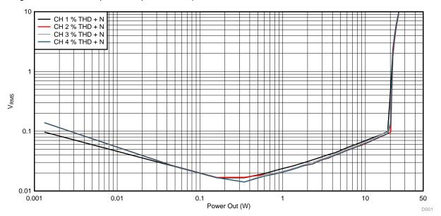
Figure 21. Power Output (W) versus THD + Noise (%)-Channels Driven Individually
