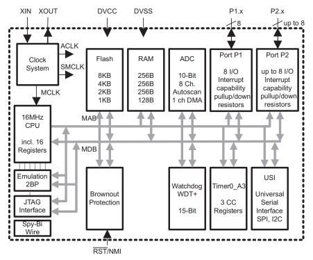
Figure 6. MSP430G2332 Functional Block Diagram
