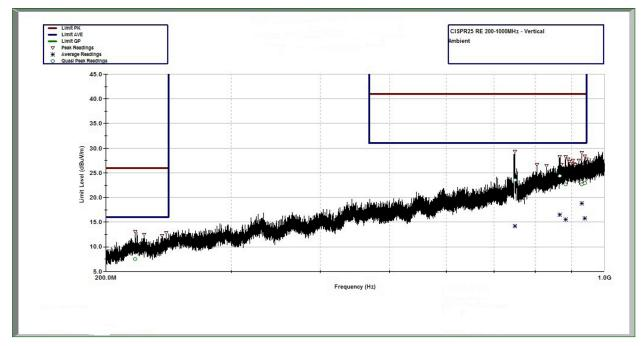
Figure 32. CISPR 25 Radiated Emissions: 200 MHz to 1 GHz, Vertical Antenna Orientation, Ambient Scan
