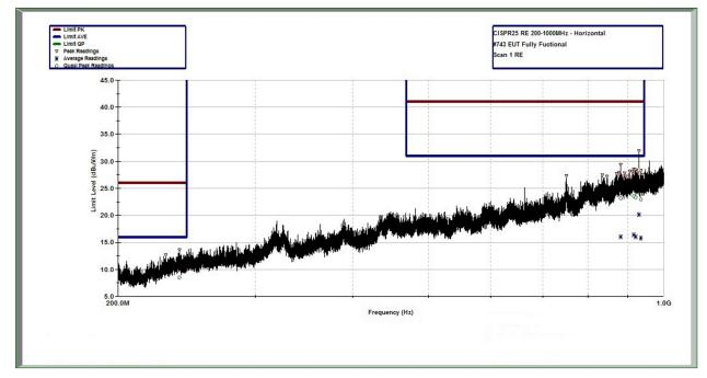
Figure 33. CISPR 25 Radiated Emissions: 200 MHz to 1 GHz, Horizontal Antenna Orientation
