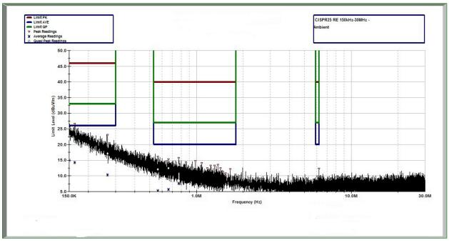
Figure 25. CISPR 25 Radiated Emissions: 150 kHz to 30 MHz, Ambient
