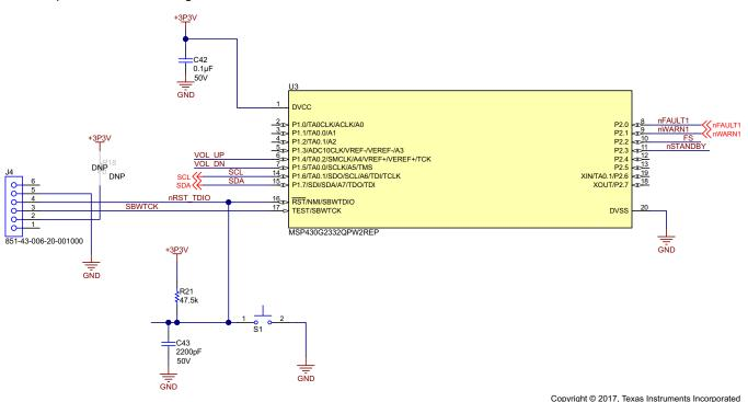
Figure 12. TIDA-00743 Microcontroller
