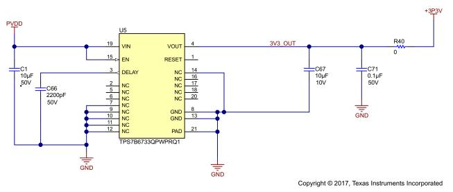
Figure 8. TPS7B6733-Q1 Linear Regulator Circuit
