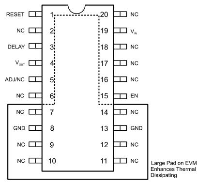
Figure 3. TPS7B6733-Q1 Enhanced Thermal Pad
