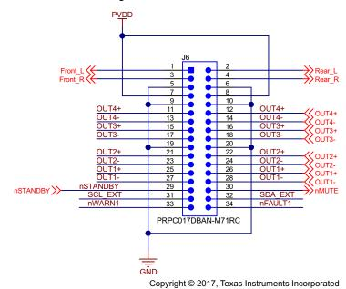
Figure 13. TIDA-00743 Interface Connector
