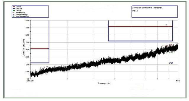
Figure 31. CISPR 25 Radiated Emissions: 200 MHz to 1 GHz, Horizontal Antenna Orientation, Ambient Scan
