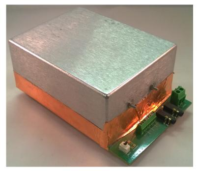
Figure 18. TIDA-00743 in Metal Box for EMI Tests
