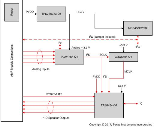
Figure 1. TIDA-00743 Block Diagram
