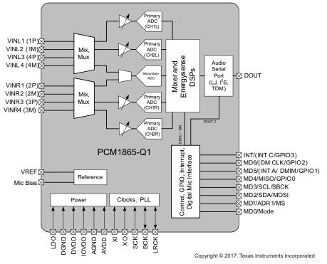
Figure 4. PCM1865-Q1 Simplified Block Diagram
