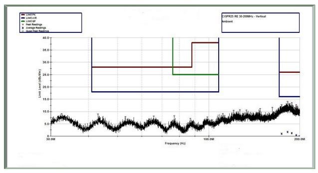
Figure 28. CISPR 25 Radiated Emissions: 30 MHz to 200 MHz, Vertical Antenna Orientation, Ambient Scan
