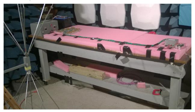
Figure 20. Radiated Emissions Test Setup
