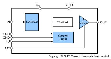
Figure 5. CDCS504-Q1 Functional Block Diagram
