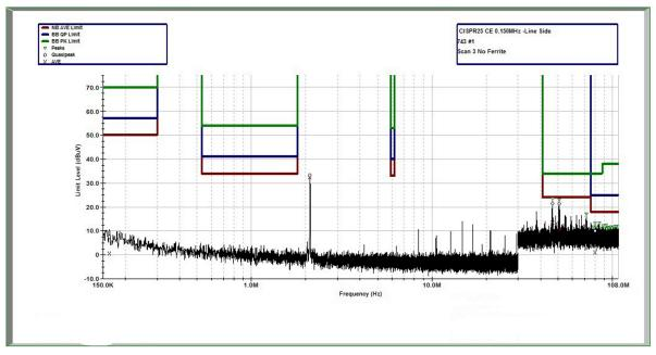
Figure 24. CISPR 25 Conducted Emissions
