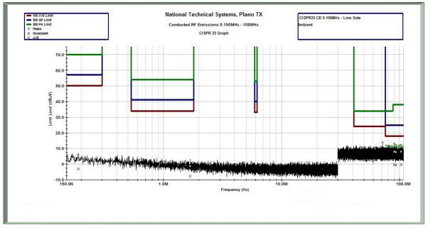
Figure 23. CISPR 25 Conducted Emissions Ambient Scan
