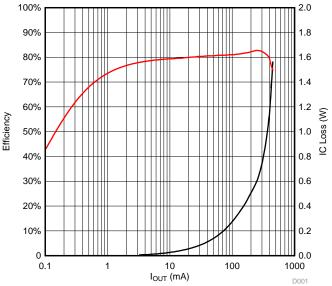
Figure 8. Efficiency Over Load (Mode = PFM)
