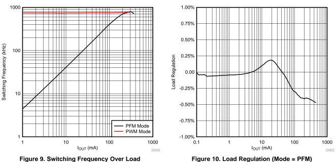
Figure 9. Switching Frequency Over Load
