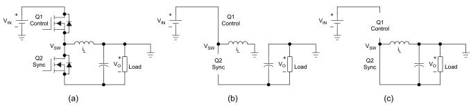
Figure 3. Inverting Buck-Boost Configuration
