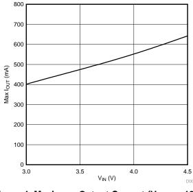
Figure 4. Maximum Output Current ( $V_{OUT} = -12 V$ )
