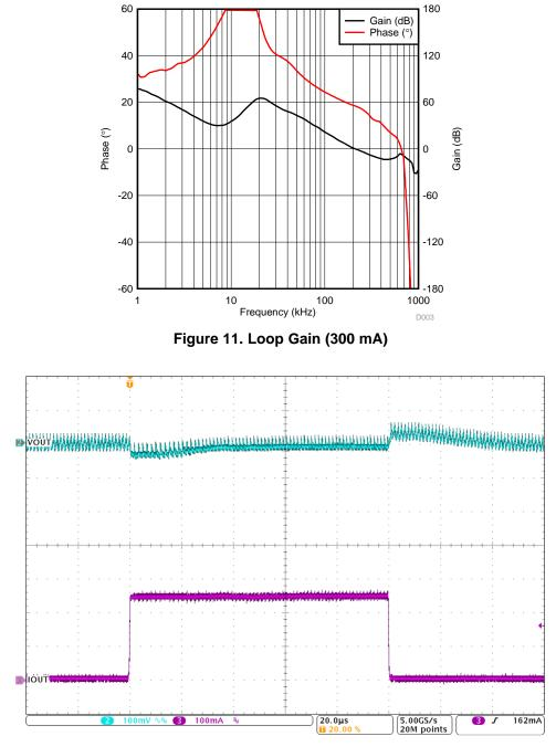
Figure 12. Transient Response (0-A to 250-mA Load Step, Mode = PWM)
