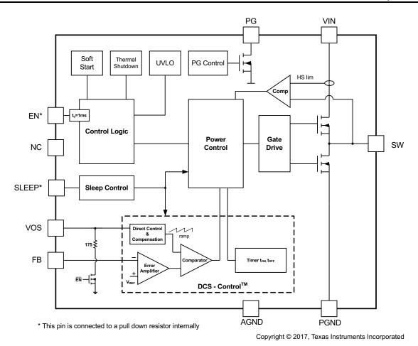
Figure 6. TPS62175 Functional Block Diagram
