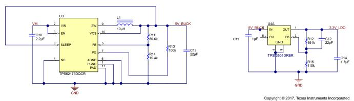
Figure 13. Board Power Management Schematic
