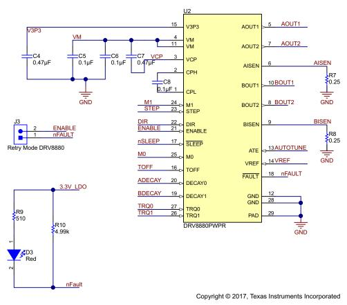
Figure 9. DRV8880 Schematic
