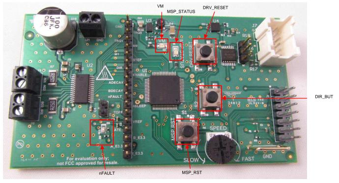
Figure 16. PCB LEDs and Push-Buttons
