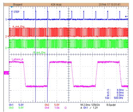
Figure 20. Current Waveform in Motor Phases Driven in Full Step Mode
