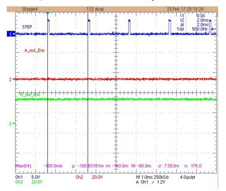
Figure 28. Encoder Outputs With 600-Resolution Encoder During Stall Condition
