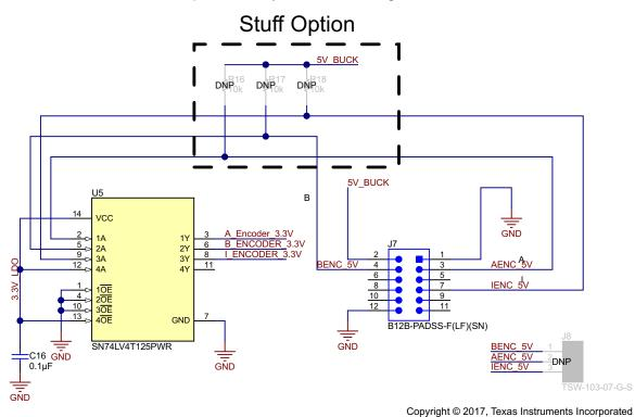
Figure 11. Encoder Header and Voltage Level Translator Schematic
