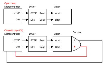
Figure 2. Open Loop versus Closed Loop Diagram
