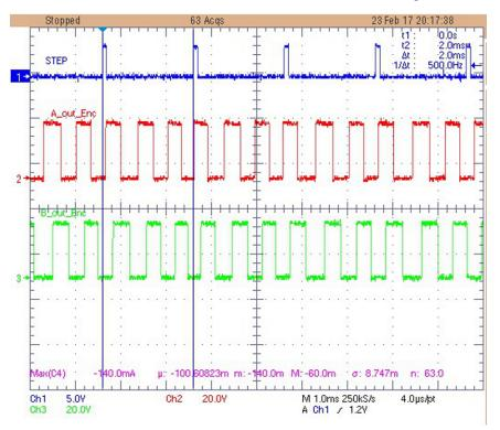
Figure 27. Encoder Outputs Using a 600-Resolution Encoder
