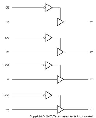
Figure 8. SN74LV4T125 Functional Block Diagram
