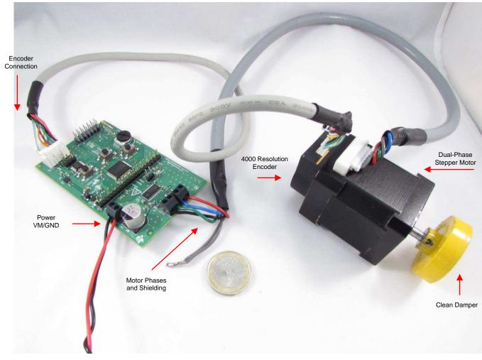
Figure 18. TIDA-01370 Board Setup With Motor
