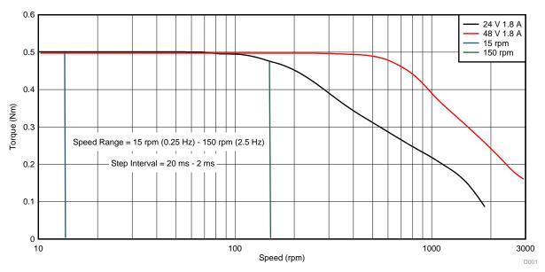
Figure 19. Motor Speed-Torque Curve
