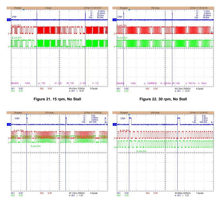
Figure 23. 75 rpm, No Stall
