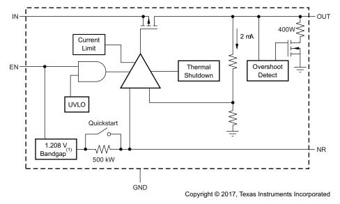
Figure 7. TPS73501 Functional Block Diagram (Fixed Output Voltage)
