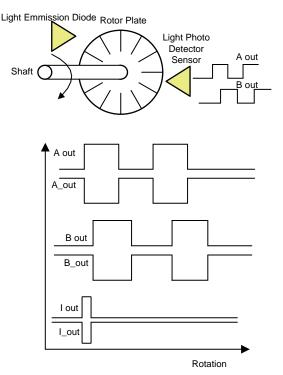
Figure 1. Encoder Structure (Above) and Encoder Outputs (Below)
