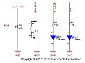
Figure 12. POT, MSP\_RST Button, STATUS, and VM LED Schematic
