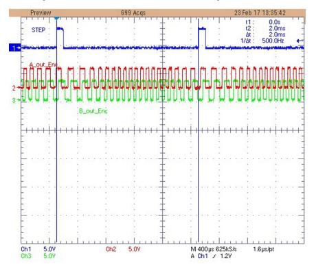
Figure 25. Zoom on A and B Patterns at Maximum Speed
