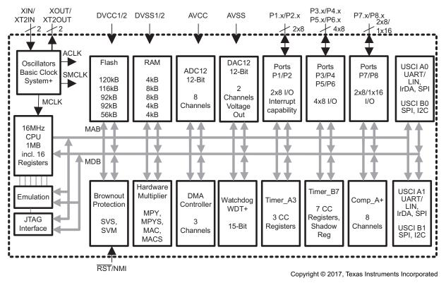
Figure 5. MSP430F2617 Functional Block Diagram
