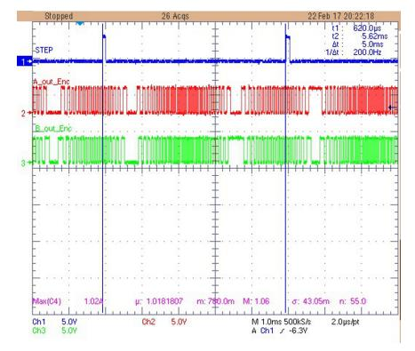
Figure 29. Resonance Condition at 5 ms
