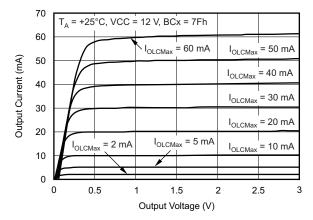
Figure 12. Residue Voltage of TLC5971
