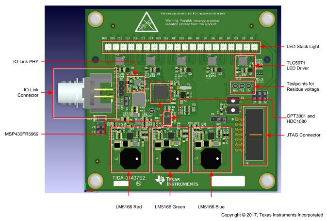
Figure 10. Subsystems of Stacklight Reference Design
