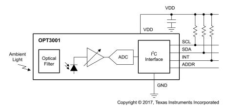
Figure 2. OPT3001 Functional Block Diagram
