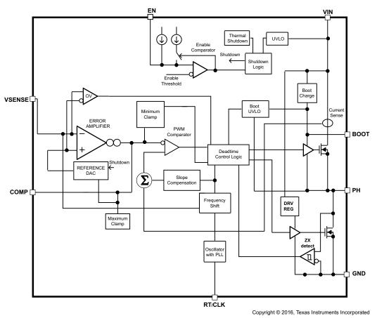
Figure 6. Block Diagram of TPS54062
