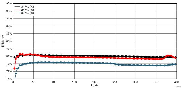
Figure 41. Efficiency of LM5166 in PFM Mode
