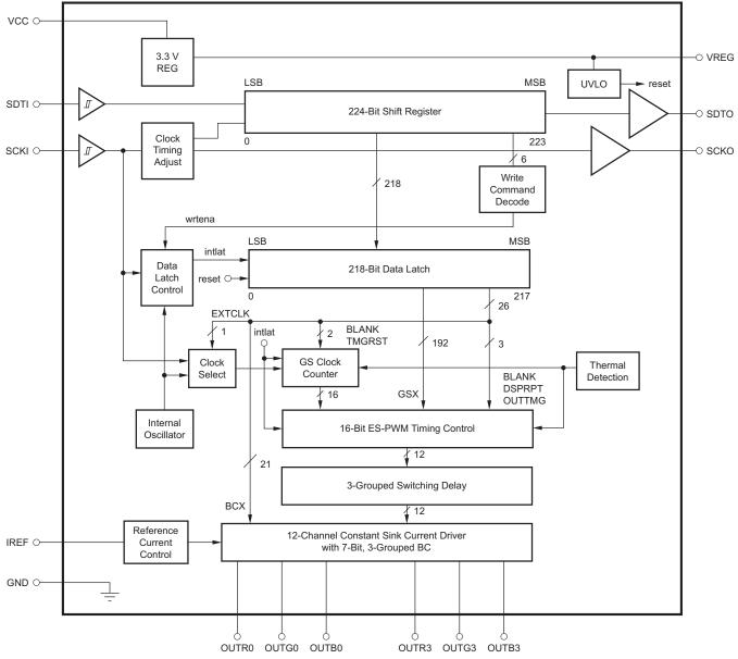
Figure 9. TLC5971 Functional Block Diagram
