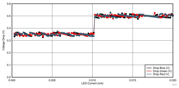
Figure 38. Voltage Drop on TLC5971 With Headroom Control
