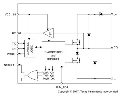
Figure 8. TIOL111 Functional Block Diagram
