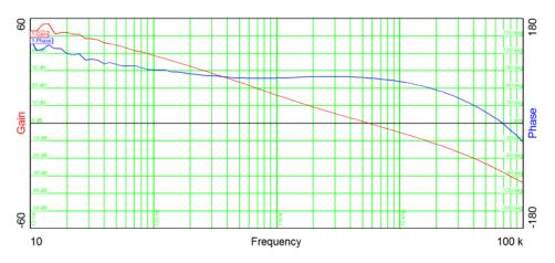
Figure 42. Loop Compensation of TPS54062
