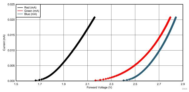
Figure 34. LED Forward Voltage
