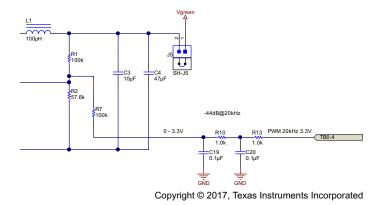
Figure 14. Schematic of Voltage Control for Voltage Regulator
