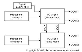
Figure 1. TIDA-01454 Block Diagram
