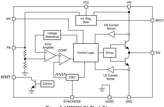
Figure 2. LM53601-Q1 Block Diagram
