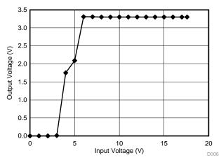
Figure 30. Buck Output Voltage Versus Input Voltage
