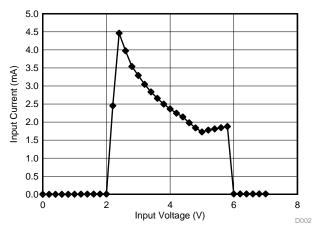
Figure 34. Boost Converter Input Current Versus Input Voltage
