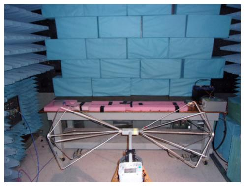
Figure 41. Biconical Antenna in Horizontal Orientation Test Setup
