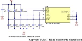
Figure 21. Input Power Filtering for Piccolo™ MCU
