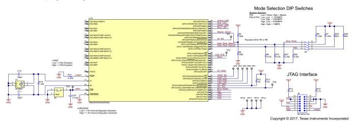
Figure 22. Mode Selection and Programming Interface Circuitry
