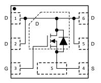
Figure 7. CSD17313Q2 Block Diagram
