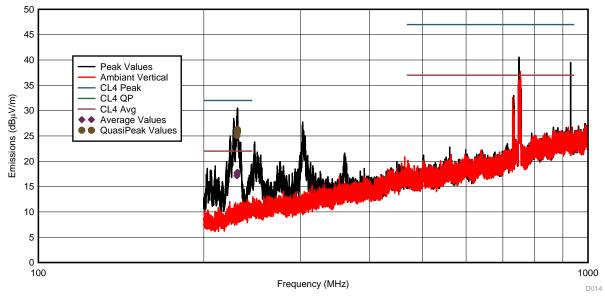
Figure 48. Vertical Logarithmic Antenna Test Results
