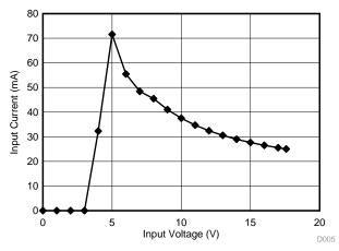
Figure 29. Buck Input Current Versus Input Voltage
