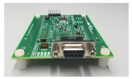
Figure 16. External Connector on PCB
