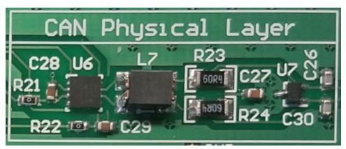
Figure 14. CAN Physical Layer Circuitry on PCB
