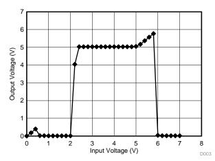
Figure 35. Boost Converter Output Voltage Versus Input Voltage
