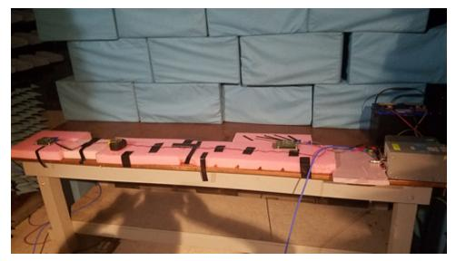
Figure 49. Conducted Emissions Setup
