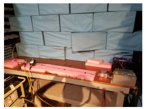
Figure 53. Bulk Current Injection Test Setup
