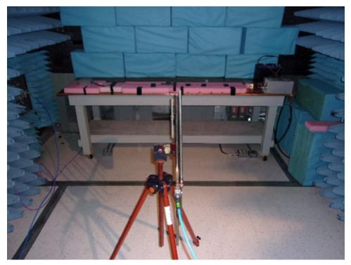
Figure 47. Logarithmic Antenna in Vertical Orientation Test Setup
