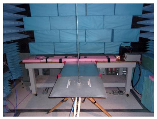
Figure 39. Dipole Antenna Test Setup
