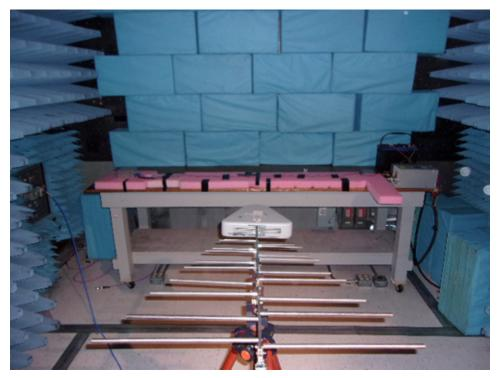
Figure 45. Logarithmic Antenna in Horizontal Orientation Test Setup
