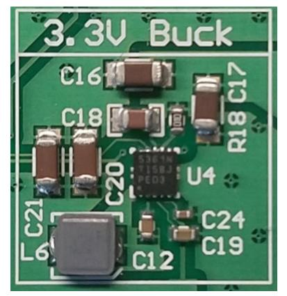
Figure 10. LM53601-Q1 Buck Converter PCB Solution Size
