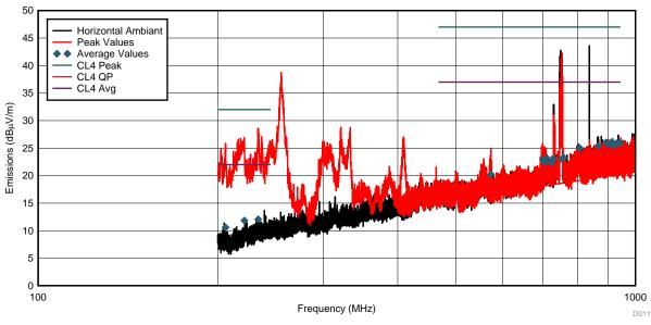
Figure 46. Horizontal Logarithmic Antenna Test Results
