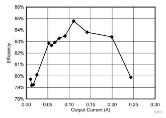
Figure 36. Boost Converter Efficiency Measurements
