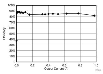
Figure 31. Buck Converter Efficiency Measurements
