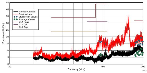
Figure 44. Vertical Biconical Antenna Test Results
