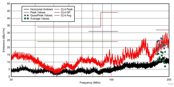
Figure 42. Horizontal Biconical Antenna Test Results
