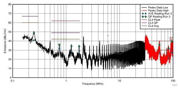
Figure 52. Conducted Emissions Results for Power Return Line
