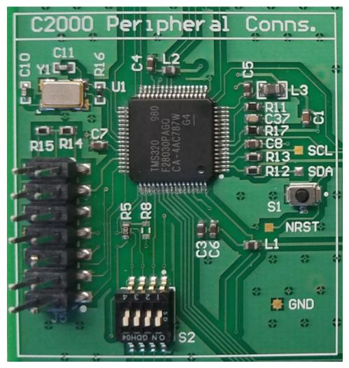
Figure 23. C2000<sup>™</sup> Peripheral Circuitry on PCB
