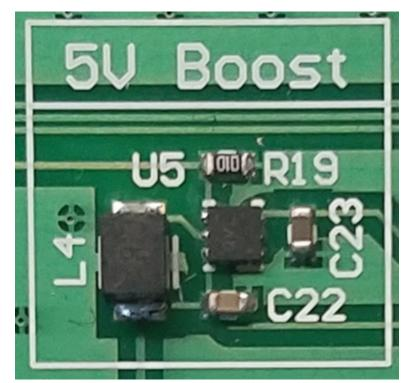
Figure 12. TPS61240-Q1 Boost Converter PCB Solution Size
