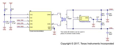
Figure 13. CAN Physical Layer Circuitry
