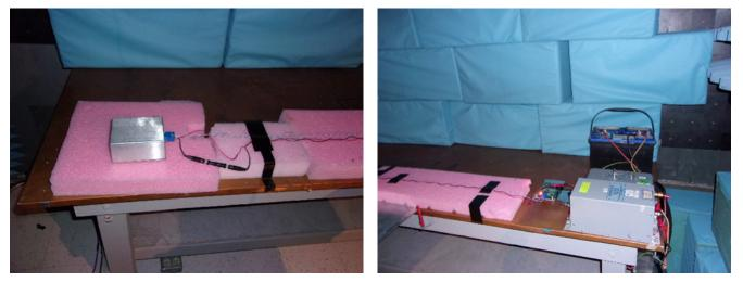
Figure 37. Slave Node Setup for RE per CISPR 25 ALSE
