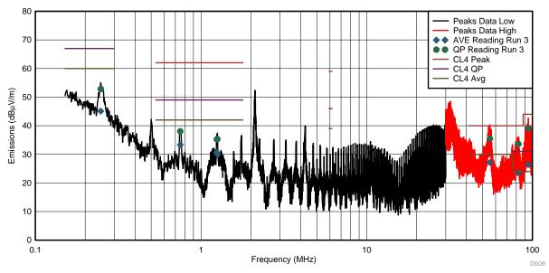
Figure 51. Conducted Emissions Results for Power Supply Line
