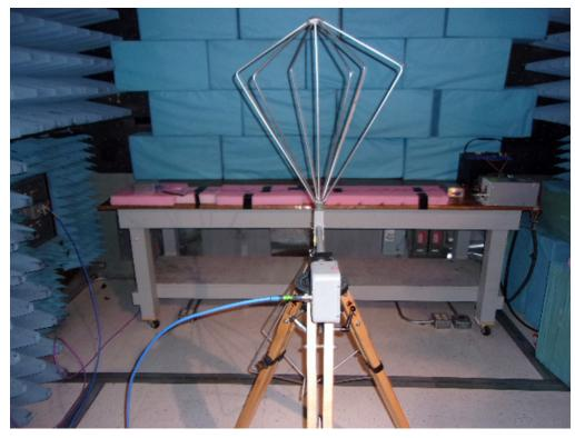
Figure 43. Biconical Antenna in Vertical Orientation Test Setup
