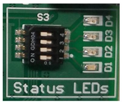
Figure 20. Status LED Circuitry on PCB
