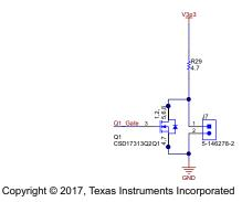
Figure 17. Dummy Load Circuitry
