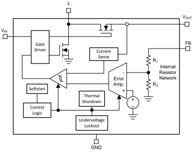
Figure 3. TPS61240-Q1 Block Diagram
