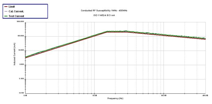
Figure 68. BCI Results With Current Injection Probe at 450 mm
