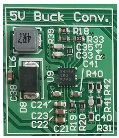
Figure 15. TPS57140-Q1 Buck Converter Circuitry on PCB
