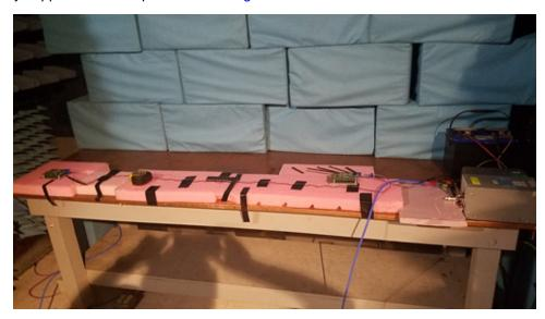
Figure 63. Conducted Emissions Setup
