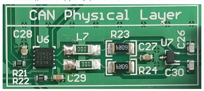
Figure 19. CAN Physical Layer Circuitry on PCB
