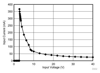
Figure 36. Boost Input Current Versus Falling Input Voltage
