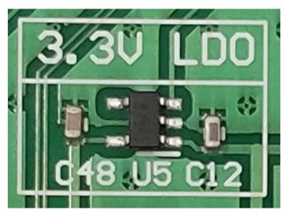
Figure 17. TLV71333P-Q1 LDO Circuitry on PCB
