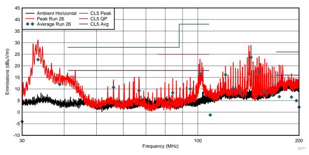
Figure 56. Horizontal Biconical Antenna Results
