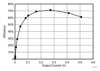
Figure 40. Boost Controller Efficiency Measurements
