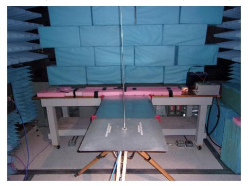
Figure 53. Radiated Emissions Dipole Antenna Setup
