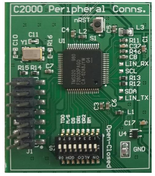
Figure 28. C2000™ Peripheral Circuitry on the PCB
