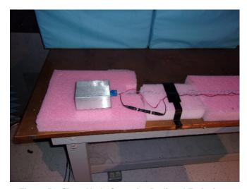
Figure 51. Slave Node Setup for Radiated Emissions
