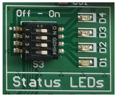
Figure 25. Status LED Circuitry on PCB
