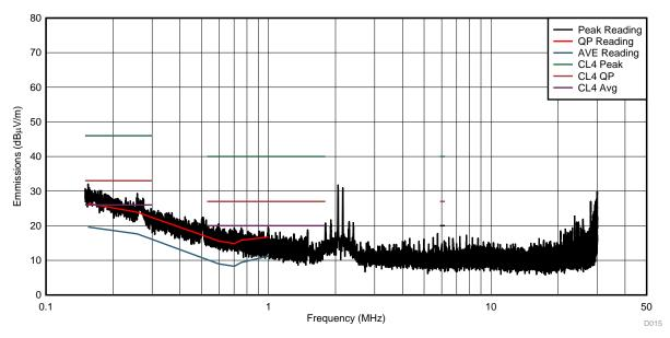
Figure 54. Radiated Emissions Dipole Antenna Results
