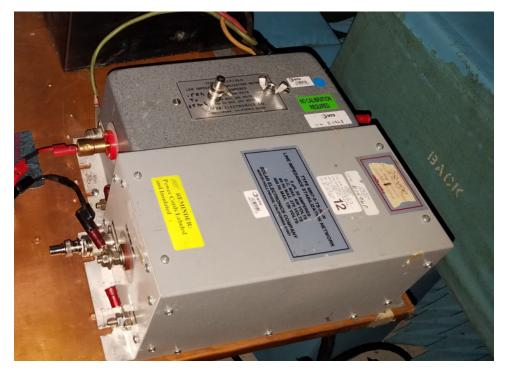
Figure 64. Artificial Networks with Measuring Ports for Conducted Emissions
