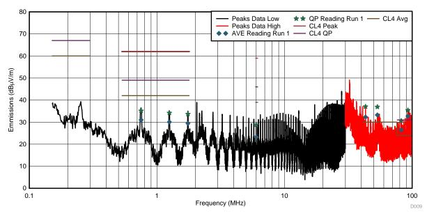
Figure 66. Conducted Emissions Results for Power Supply Return Line
