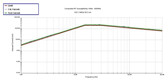
Figure 69. BCI Results With Current Injection Probe at 750 mm
