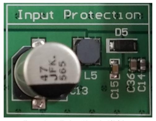
Figure 11. Battery Filtering and Protection PCB Snippet
