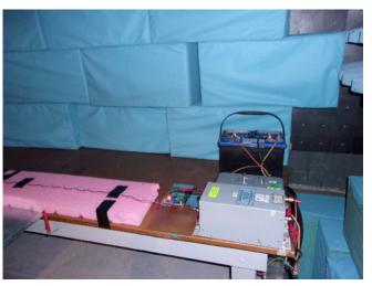
Figure 52. Master Node Setup for Radiated Emission
