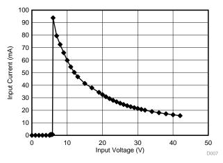
Figure 42. Buck Converter Input Current Versus Input Voltage
