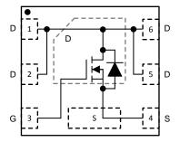
Figure 9. CSD17313Q2 Block Diagram
