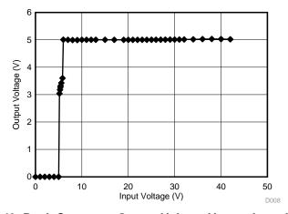
Figure 43. Buck Converter Output Voltage Versus Input Voltage
