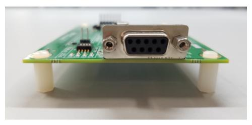
Figure 21. External Connector for Power and CAN on PCB
