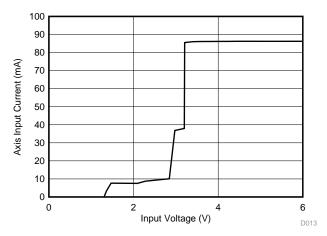
Figure 49. LDO Input Current Versus Input Voltage
