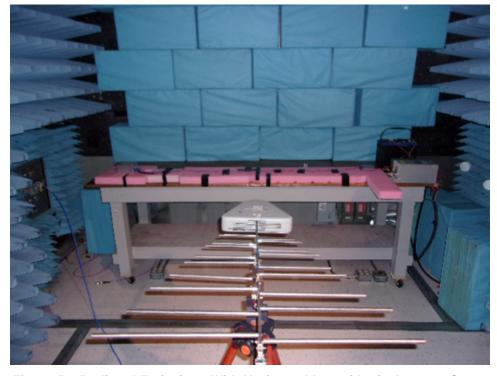
Figure 59. Radiated Emissions With Horizontal Logarithmic Antenna Setup
