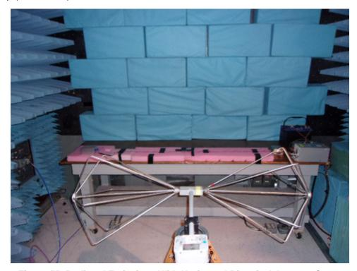
Figure 55. Radiated Emissions With Horizontal Biconical Antenna Setup
