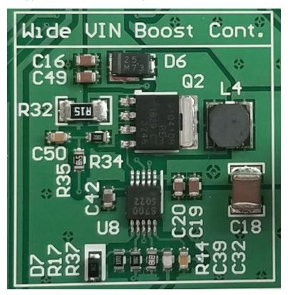
Figure 13. LM5022-Q1 Boost Controller Circuitry on PCB
