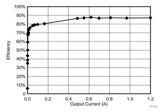
Figure 44. Buck Converter Efficiency Measurements
