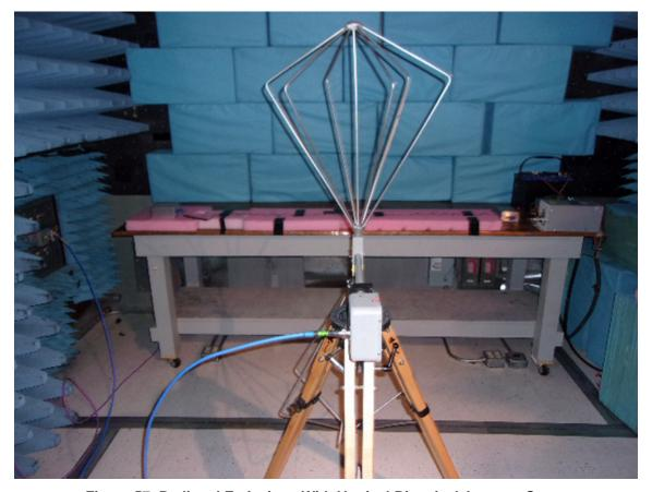
Figure 57. Radiated Emissions With Vertical Biconical Antenna Setup
