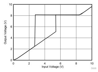
Figure 38. Boost Output Voltage Versus Low Input Voltages
