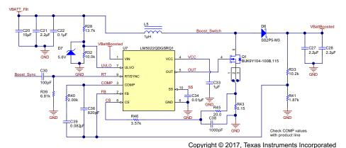
Figure 12. LM5022-Q1 Non-Synchronous Boost Controller Circuitry
