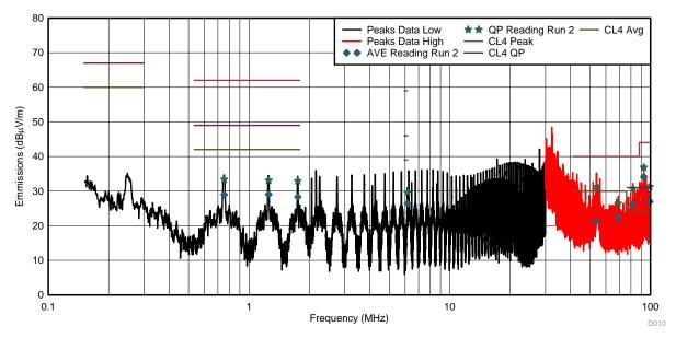
Figure 65. Conducted Emissions Results for Power Supply Line
