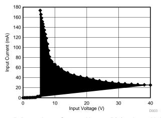
Figure 35. Boost Input Current Versus Rising Input Voltage
