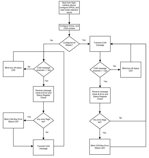
Figure 33. Program Flow Diagram
