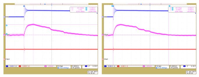
Figure 47. Buck Converter Load Step Decrease Response
