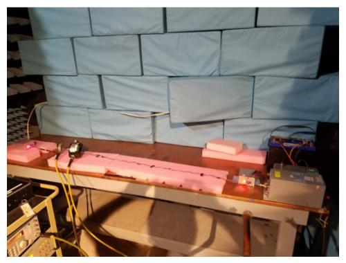
Figure 67. Bulk Current Injection Test Setup
