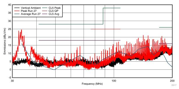
Figure 58. Vertical Biconical Antenna Results
