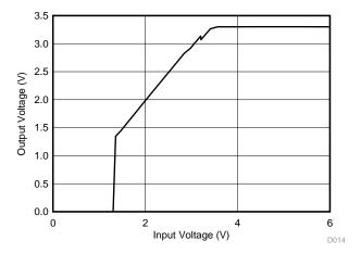
Figure 50. LDO Output Voltage Versus Input Voltage
