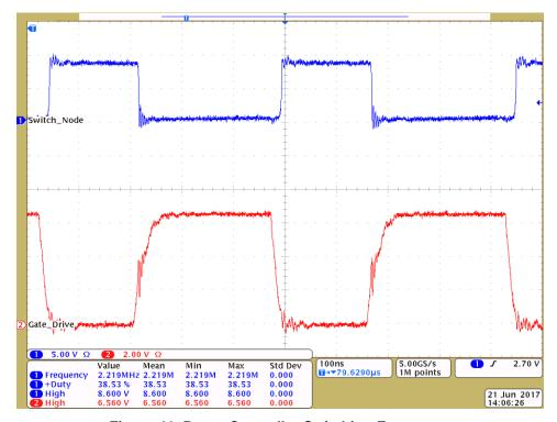
Figure 41. Boost Controller Switching Frequency
