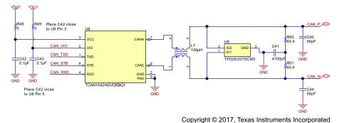
Figure 18. TCAN1042V-Q1 CAN Physical Layer Circuitry
