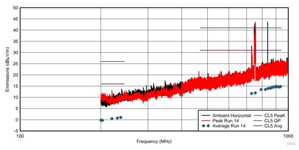
Figure 60. Horizontal Logarithmic Antenna Results
