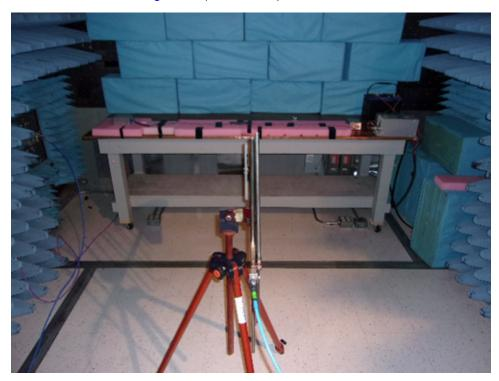
Figure 61. Radiated Emissions With Vertical Logarithmic Antenna Setup
