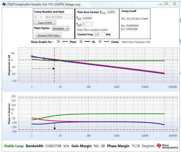
Figure 3-26. Voltage Loop PI Compensation Tuning Using Compensation Designer
