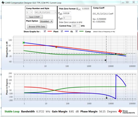
Figure 3-14. Current Loop Design Using Compensation Designer
