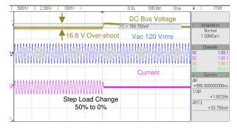
Figure 3-61. Voltage Transient With Non-Linear Voltage Loop, Vin 120 Vrms, 880 W to 0 W Transient, Overshoot 16.8 V
