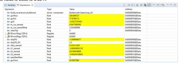
Figure 3-34. Lab 6 Watch Expression Showing Measured Voltage and Currents
