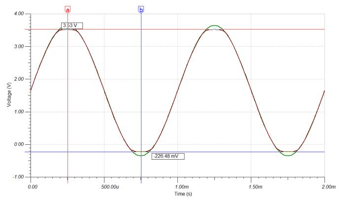
Figure 10. Overvoltage Clipping by Input Protection Diodes
