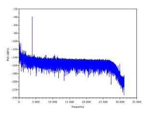
Figure 28. PSD for -37-dBFS Input at 3.9 kHz
