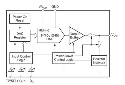
Figure 6. DAC5311 Block Diagram
