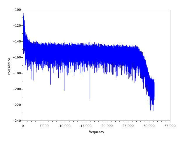
Figure 27. Noise Floor With XTR111 Enabled
