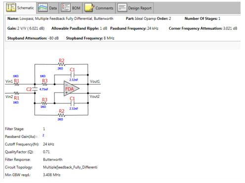
Figure 9. Filter Design Using TI FilterPro<sup>™</sup> Tool
