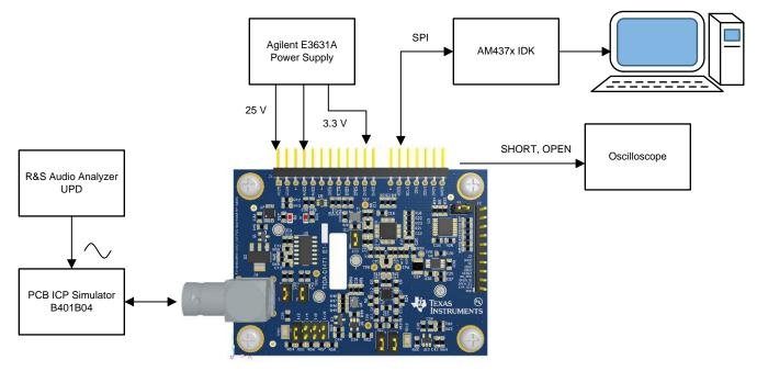
Figure 20. TIDA-01471 Test Setup
