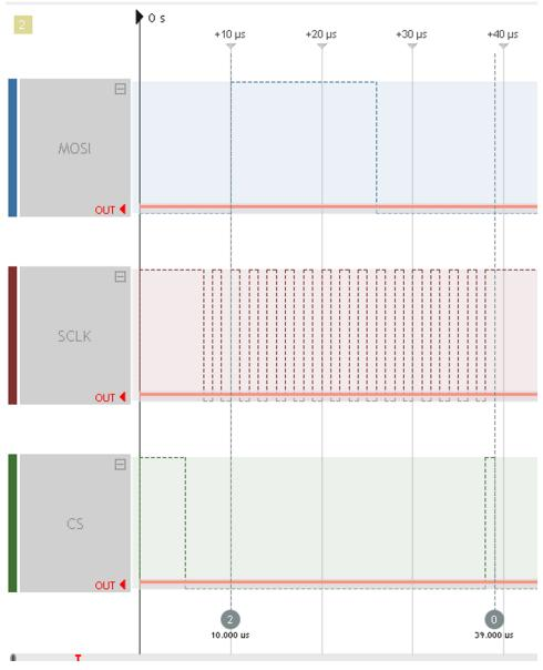
Figure 11. Example SPI Waveform for DAC5311 Programming
