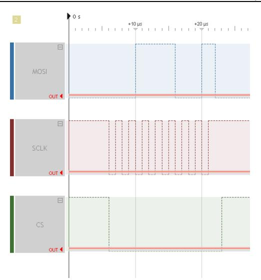
Figure 12. Example SPI Waveform for SN74HC595 Programming
