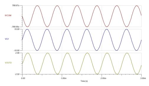
Figure 18. Output Current of VCOM Reference
