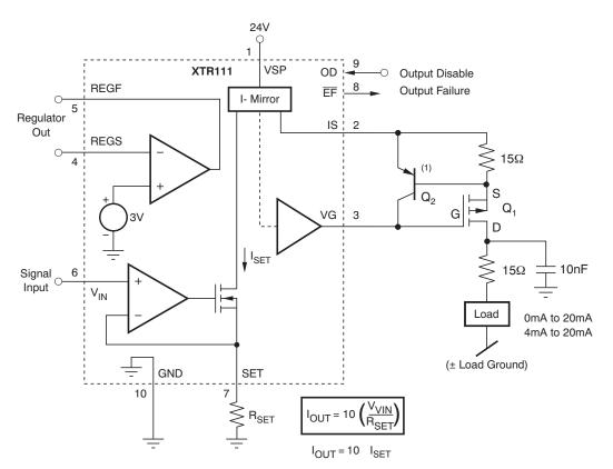
Figure 5. XTR111 Block Diagram
