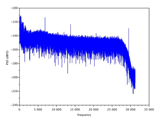
Figure 25. Noise in Presence of Image Frequency at 8.01 MHz
