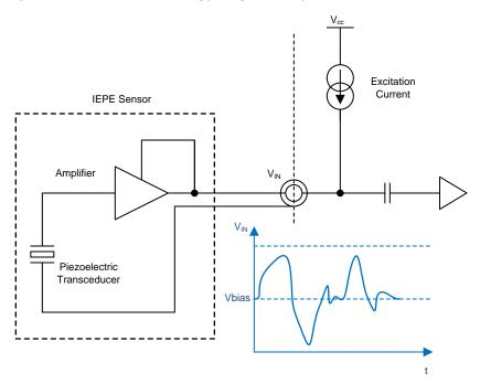
Figure 7. IEPE Sensor Conceptual Circuit
