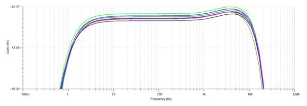
Figure 14. Signal Chain Passband at –12-dB Gain Setting
