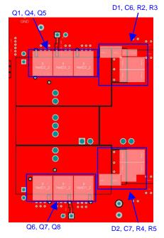
Figure 44. Placement of Synchronous Rectification MOSFETs and Snubber Circuit
