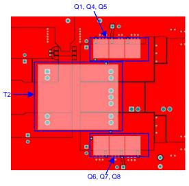
Figure 43. Synchronous Rectification MOSFETs and Power Transformer T2
