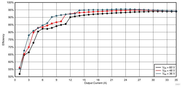
Figure 28. Measured Efficiency Under Input Voltages of 36 V, 48 V, and 60 V
