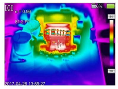
Figure 34. Thermal Image of Primary Side Switches (Q2, Q9, Q3, and Q10)
