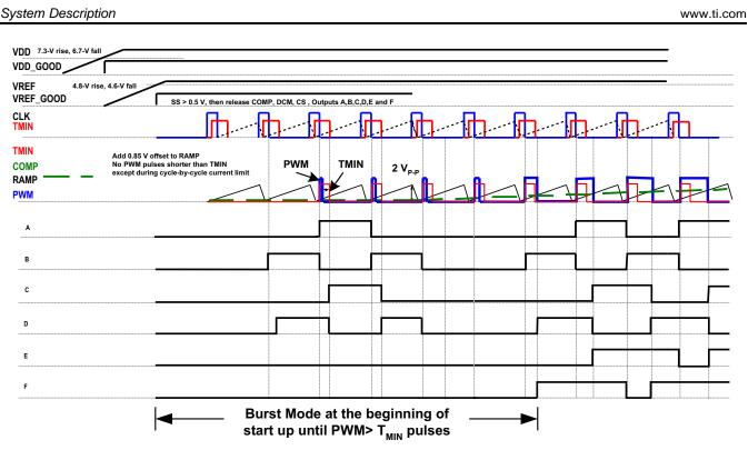
Figure 11. UCC28951-Q1 Start-Up Waveform and Burst Mode Operation
