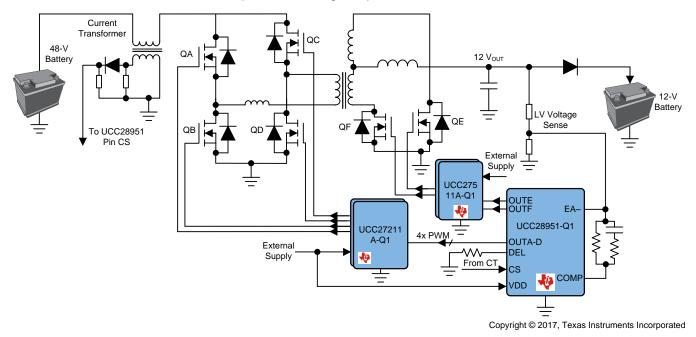
Figure 2. TIDA-01407 Block Diagram
