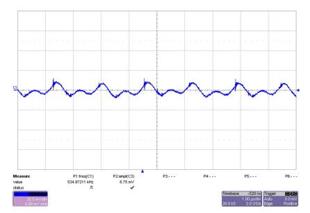
Figure 18. Output Voltage Ripple of TIDA-01407 With  $V_{IN}$  = 48 A and  $I_{OUT}$  = 33.3 A
