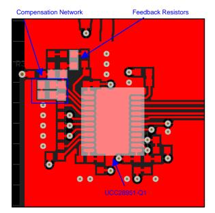
Figure 47. Placement of Compensation Network
