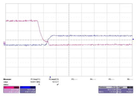
Figure 20. Switch Node CD (SW\_CD) and Gate Drive D
