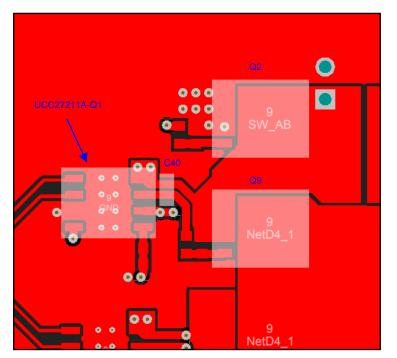
Figure 45. Placement of Gate Driver and MOSFETs at Converter Primary Side
