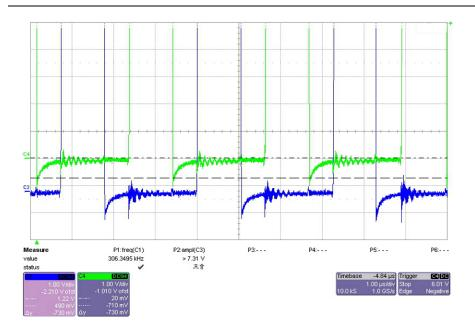
**NOTE:** From top to bottom: CH4 – Switch node voltage of Q6, CH3 – Switch node voltage of Q1
