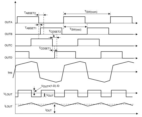
Figure 10. PWM Control and Output Waveforms of Phase-Shifted Full-Bridge Converter
