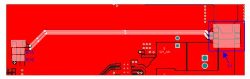
Figure 42. Placement of RC Filtering Network for Current Sense Pin (PCB Top Side)
