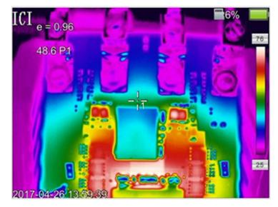
Figure 36. Thermal Image of Secondary Side Synchronous Rectifier (Q1, Q4, Q5, Q6, Q7, and Q8)
