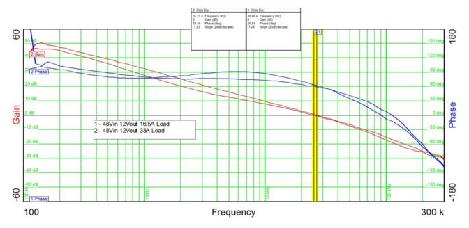
Figure 38. Loop Frequency Response of TIDA-01407 With V<sub>IN</sub> = 48 V and 16.5-A Load and 33-A Load
