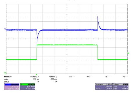
Figure 33. Load Transient Response With  $V_{IN}$  = 48 V and  $I_{OUT}$  Switching Between 33 A and 16.5 A
