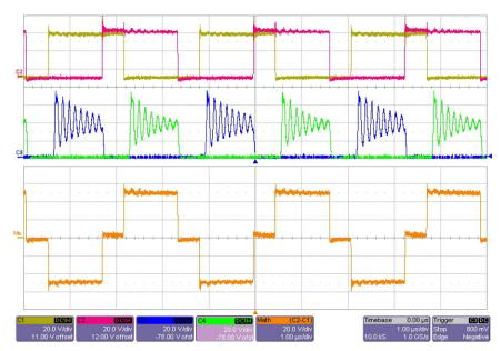
Figure 30. Switch Node Voltages and Voltage Across Transformer Primary Winding Under V<sub>IN</sub> = 48 V,  $I_{OUT}$  = 33 A
