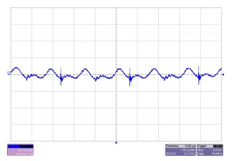
Figure 17. Output Voltage Ripple of TIDA-01407 With  $V_{IN}$  = 48 V and  $I_{OUT}$  = 15 A
