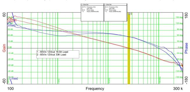
Figure 39 shows the loop frequency response with a 60-V input voltage, 16.5-A load, and 33-A load, respectively. As the graph show, phase margins of 57.63° and 58.35° are achieved, respectively.
