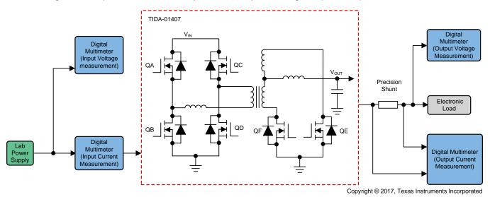
Figure 27. Experiment Setup of Efficiency Measurement
