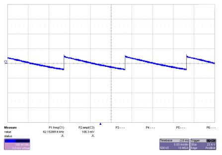
Figure 16. Output Voltage Ripple of TIDA-01407 With  $V_{IN}$  = 48 A and No Load
