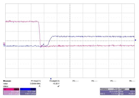
Figure 24. Switch Node CD (SW\_CD) and Gate Drive D
