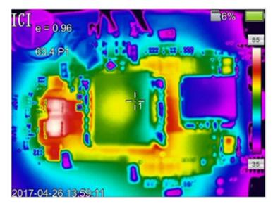
Figure 35. Thermal Image of Power Transformer T2
