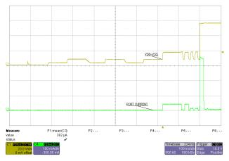
Figure 25. PoE Class and Detection
