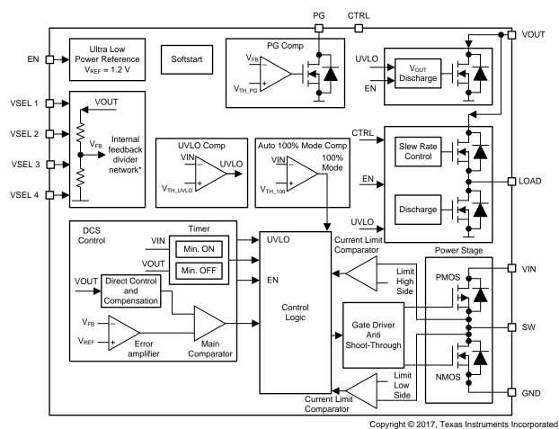
Figure 5 shows the TPS62740 block diagram.
