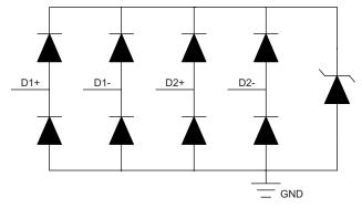
Figure 8. TPD4E05U0-Q1 Block Diagram
