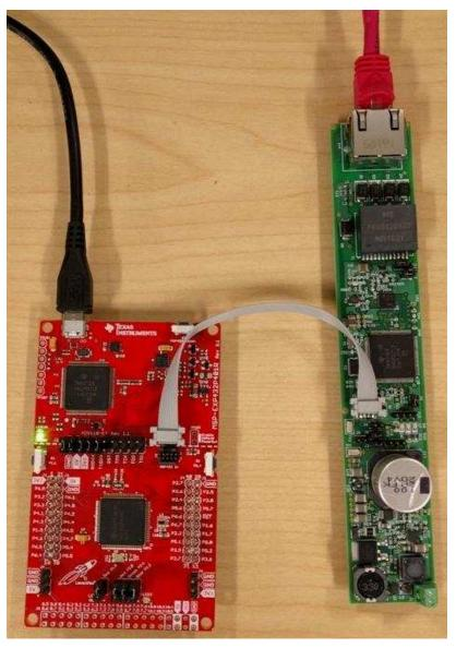
Figure 16. PCB Connected to XDS110-ET on LaunchPad
