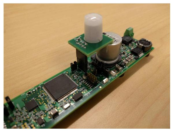
Figure 20. TIDA-01463 PCB With IR Sensor Attached
