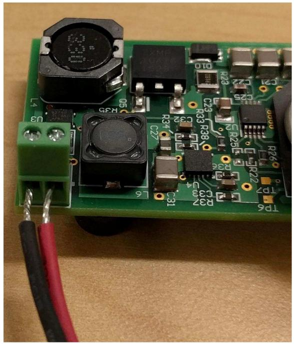
Figure 21. TIDA-01463 LED Output Connection on PCB
