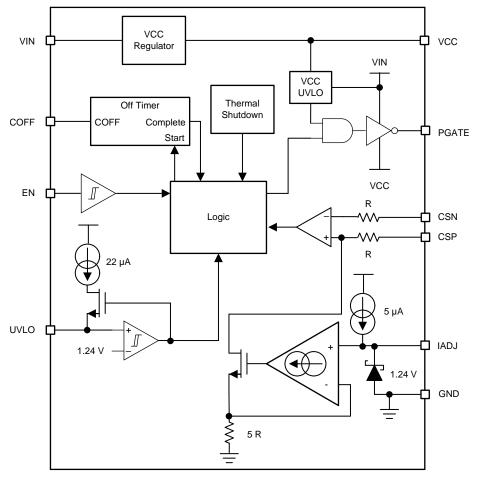
Figure 3. LM3409HV Block Diagram
