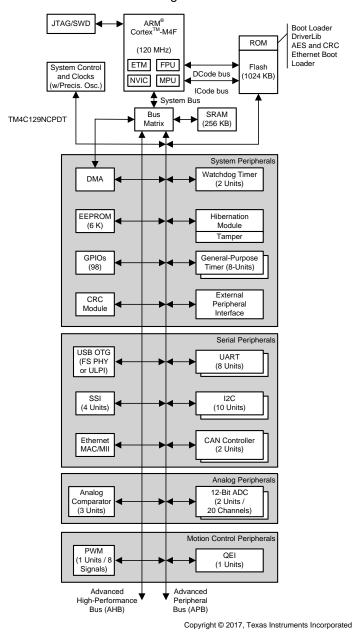
Figure 6 shows the TM4C1292NCPDT block diagram.
