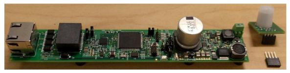
Figure 9. TIDA-01463 PCB With IR Sensor
