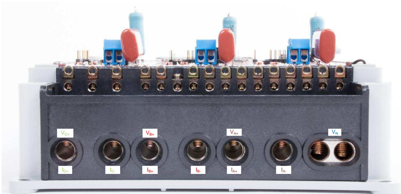
**Figure 21. Front View of EVM With Test Setup Connections**
