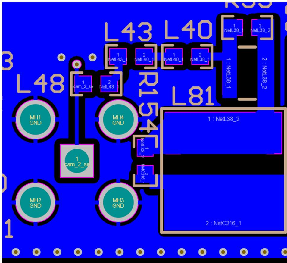
Figure 21. Power Over Coax DC Current Path
