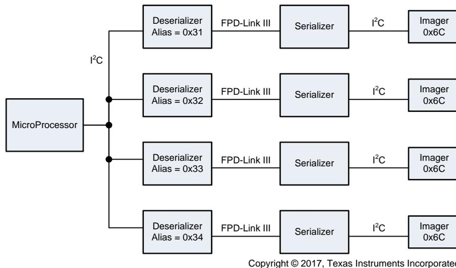
**Figure 4. I<sup>2</sup>C Address Aliasing**
