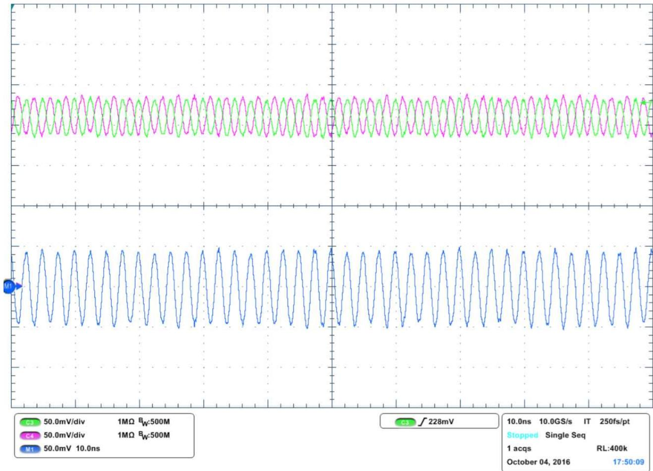
Figure 16. CSI-2 Positive and Negative Differential Voltages Measured
