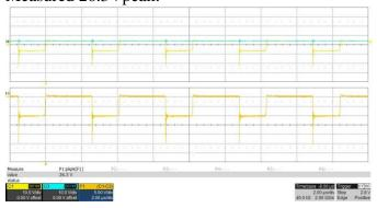
Vds, Q2, 5V/div, 2usec/div, 57VDC input, 2.9A load, 750MHz bandwidth Measured 16.3Vpeak:
