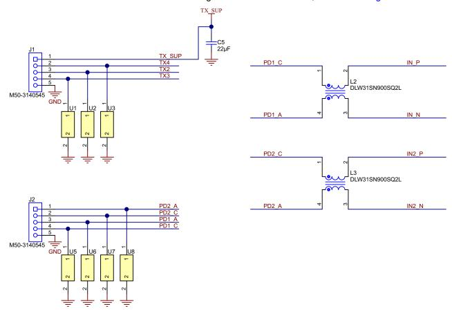
Figure 2-8. PPG Connection From Sensor Board to AFE4900 Device on Main Board
