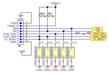
Figure 2-5. MCU Programming Connector
