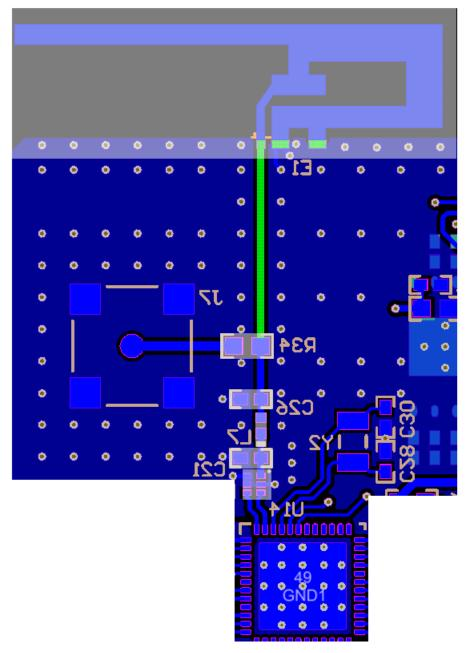
Figure 4-9. Traces Between CC2640R2F and Antenna
