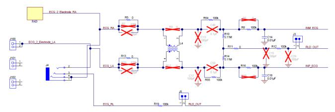
Figure 2-10. Interface for ECG Measurement (Three Electrodes)
