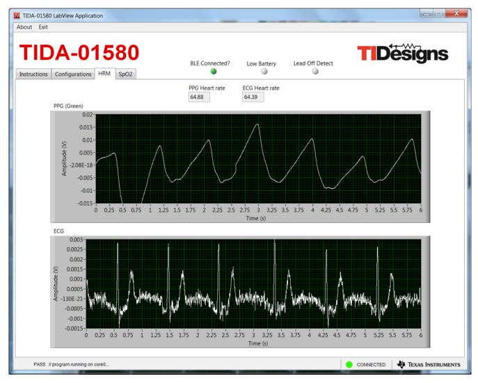
Figure 3-25. HRM Data From OCS112 Sensor and ECG Data
