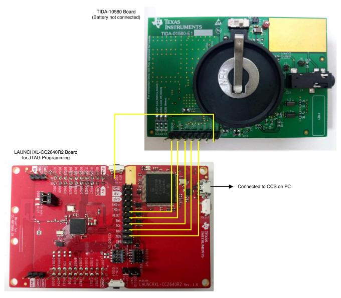
Figure 3-10. Connections Between TIDA-01580 Board and LAUNCHXL-CC2640R2
