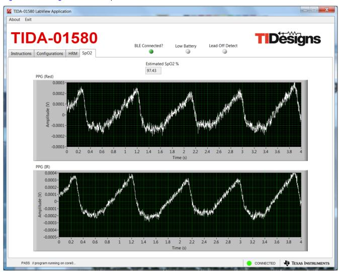
Figure 3-26. SpO2 Data From SFH 7072 Sensor and ECG Data
