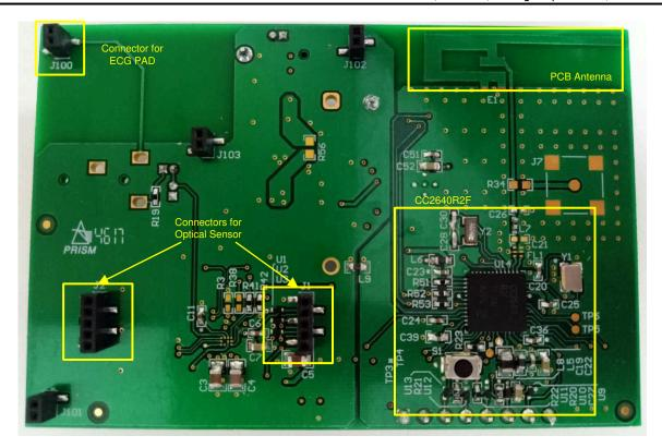
Figure 3-2. TIDA-01580 PCB - Bottom View
