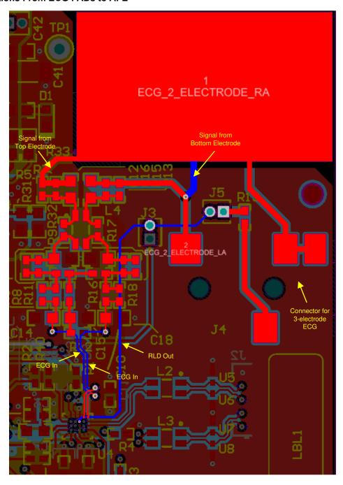
Figure 4-7. Traces From ECG PADs to AFE
