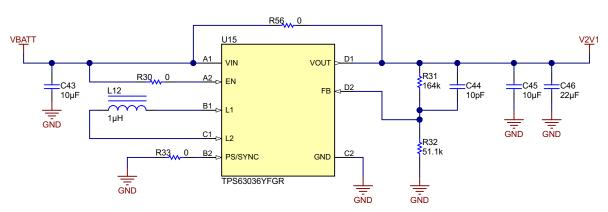
Figure 2-14. TPS63036 Buck-Boost Converter (V<sub>OUT</sub> = 2.1 V)
