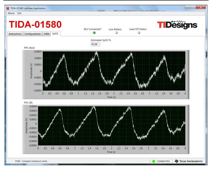
Figure 3-27. SpO2 Data From OCS112 Sensor and ECG Data
