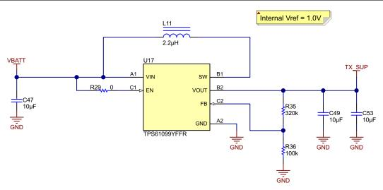
Figure 2-11. TPS61099 Boost Converter (V<sub>OUT</sub> = 4.2 V)
