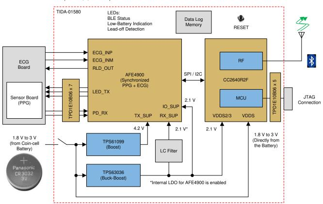
Figure 2-1. TIDA-01580 Block Diagram
