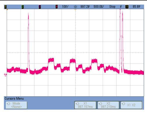
Figure 3-34. Three Pulses Showing Standard Advertising for BLE
