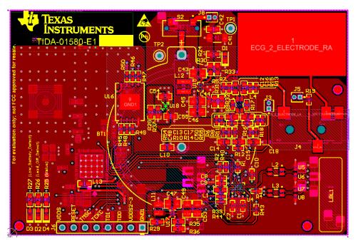
Figure 4-1. Top Layer for TIDA-01580 Board
