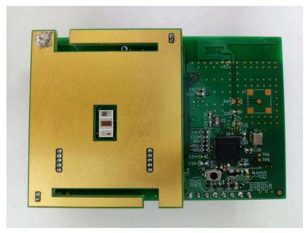
Figure 3-3. ECG and PPG Board Mounted on Main Board (Top View)
