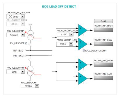
Figure 3-30. Settings for DC Lead-Off Detection
