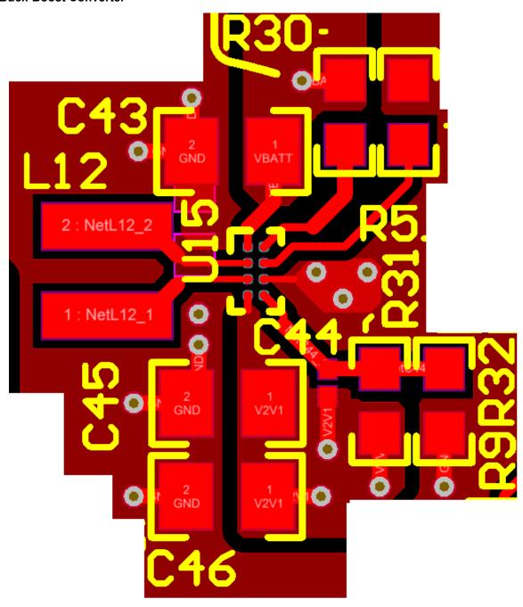
Figure 4-11. Layout and Traces for Buck-Boost Converter, TPS63036
