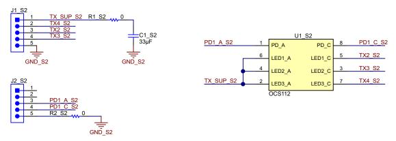
Figure 2-7. Sensor Board Schematic With OCS112 Device
