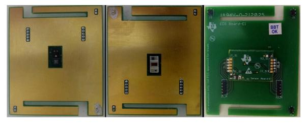
Figure 3-5. ECG and PPG Board
