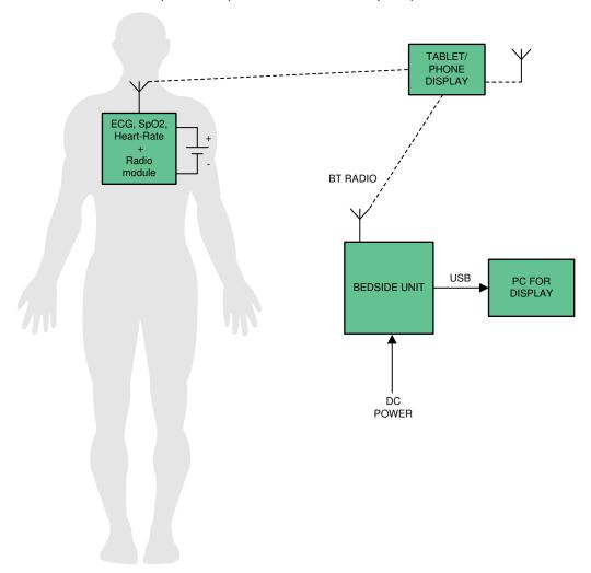
Figure 1-2. System-Level Block Diagram
