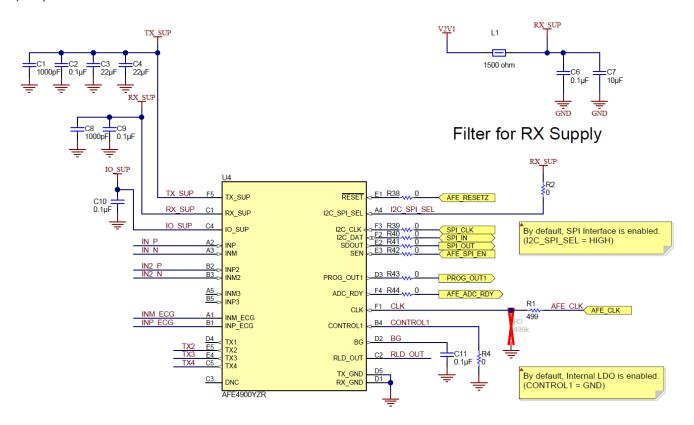
Figure 2-2. AFE4900 Connections Schematic
