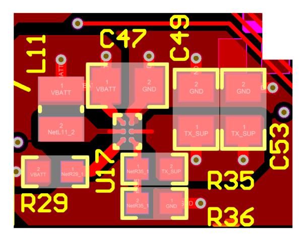
Figure 4-10. Layout and Traces for Boost Converter, TPS61099
