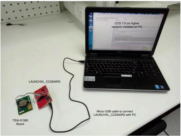
Figure 3-9. Programming TIDA-01580 Board Using LAUNCHXL-CC2640R2
