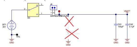
Figure 2-18. Battery Connector and Reservoir
