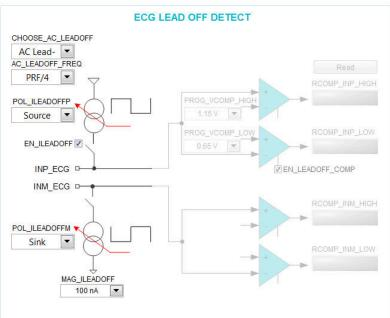
Figure 3-29. Settings for AC Lead-Off Detection
