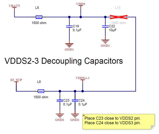
Figure 2-4. Decoupling for CC2640R2F MCU
