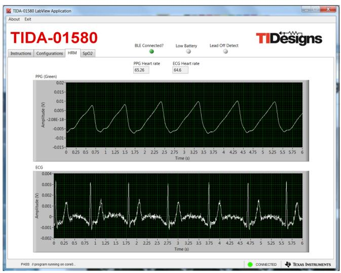
Figure 3-24. HRM Data From SFH 7072 Sensor and ECG Data
