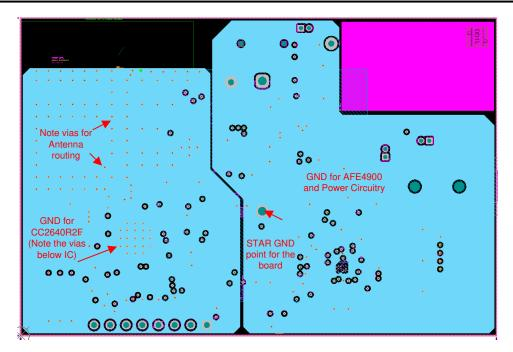
Figure 4-4. Ground Layer for TIDA-01580 Board
