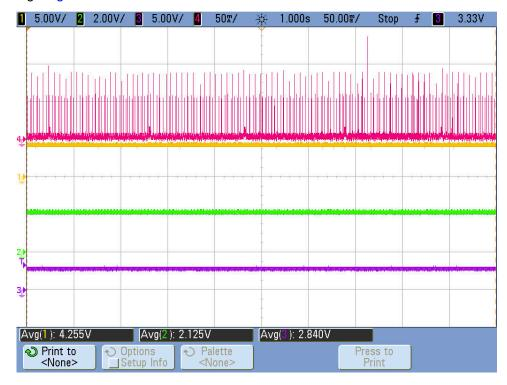
Figure 3-31. Waveform Showing Ibattery (Pink), RX\_SUP (Yellow), TX\_SUP (Green), and Vbattery (Purple)
