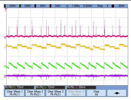
Figure 3-32. Waveform Showing Ibattery (Pink), Ripple on RX\_SUP (Yellow), Ripple on TX\_SUP (Green), and Ripple on Vbattery (Purple)
