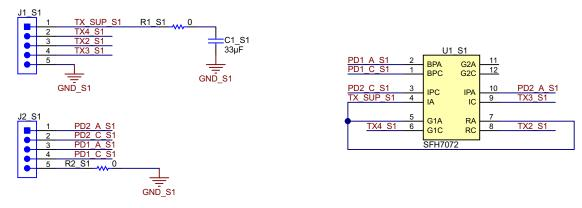
Figure 2-6. Sensor Board Schematic With SFH7072 Device
