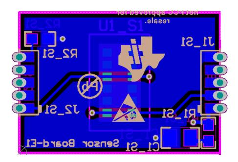
Figure 4-13. Layout for SFH 7072 Board (Bottom Layer)
