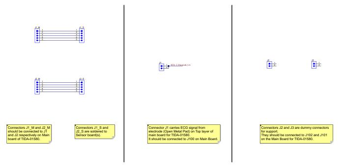
Figure 2-22. Connections Between Sensor Board and ECG Board
