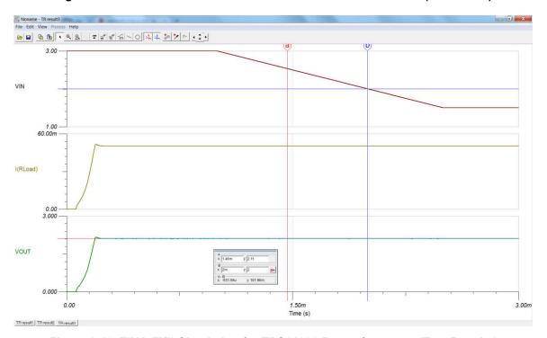
Figure 2-16. TINA-TI™ Simulation for TPS61099 Boost Converter (Test Results)
