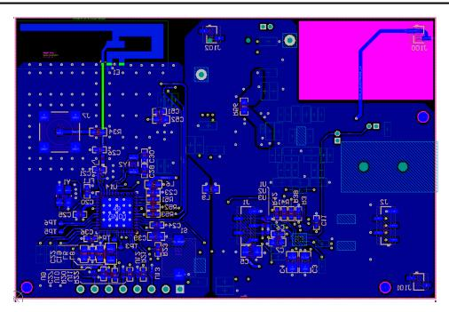
Figure 4-2. Bottom Layer for TIDA-01580 Board
