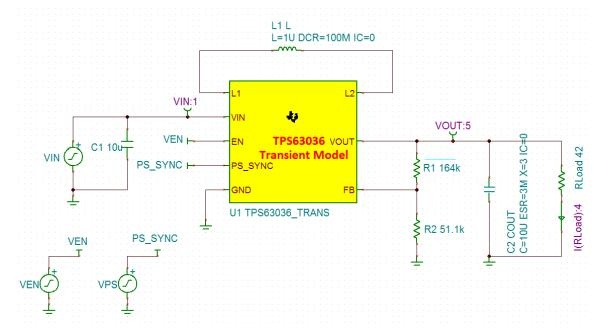
Figure 2-15. TINA-TI™ Simulation for TPS61099 Boost Converter (Schematic)
