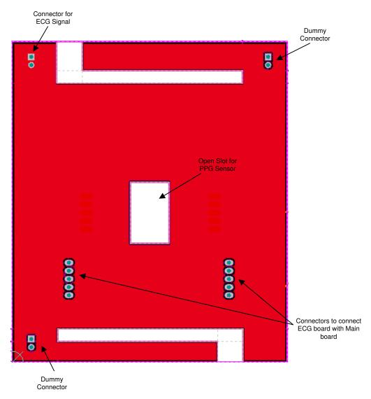
Figure 4-16. Layout for ECG Board (Top Layer)
