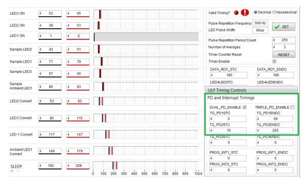
Figure 3-8. Timing and Settings for OCS112 PPG Sensor
