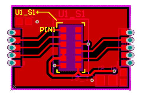
Figure 4-12. Layout for SFH 7072 Board (Top Layer)
