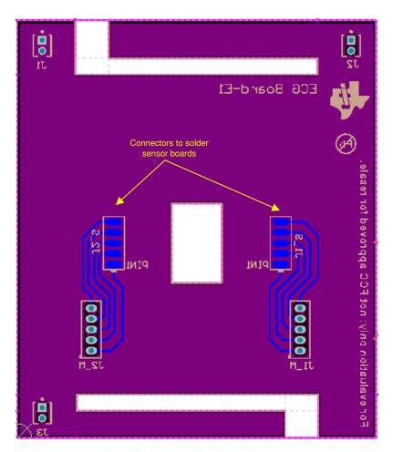
Figure 4-17. Layout for ECG Board (Bottom Layer)
