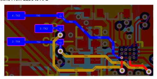
Figure 4-6. Traces From LEDs to AFE
