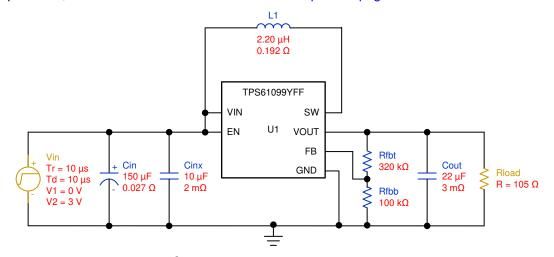
Figure 2-12. WEBENCH® Simulation for TPS61099 Boost Converter (Schematic)
