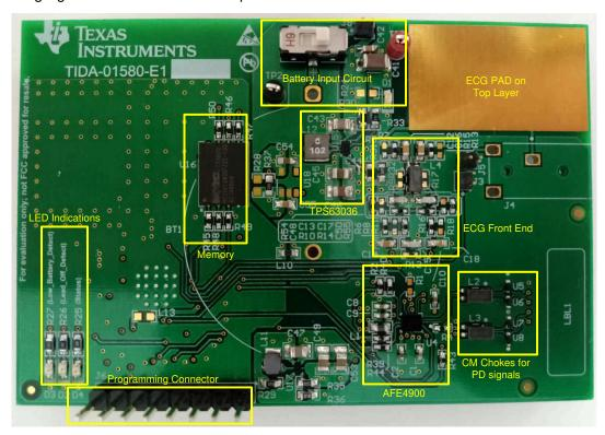
Figure 3-1. TIDA-01580 PCB - Top View Battery Holder (BT1) Not Mounted
