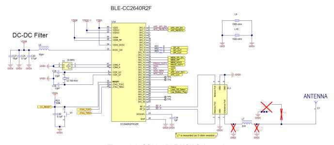
Figure 2-3. CC2640R2F MCU Schematic
