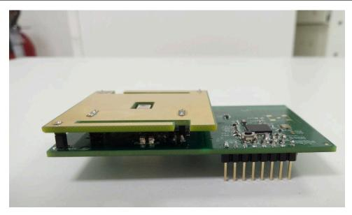
Figure 3-6. ECG and PPG Board Mounted on Main Board (Side View)
