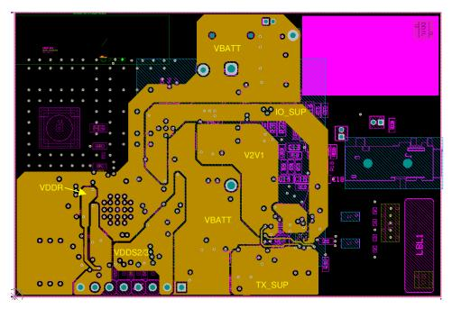
Figure 4-3. Power Layer for TIDA-01580 Board
