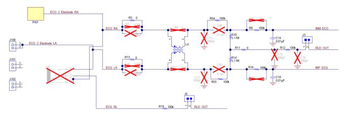
Figure 2-9. Interface for ECG Measurement (Two Electrodes)
