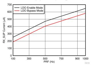
Figure 2-19. Current Consumption for AFE4900 in LDO Enable Mode
