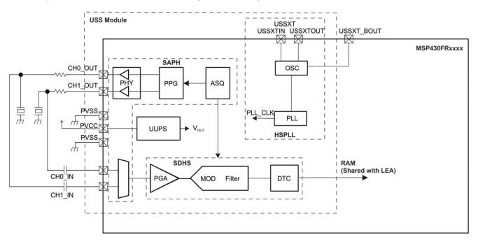
Figure 17. Ultrasonic-Sensing Solution Functional Block Diagram
