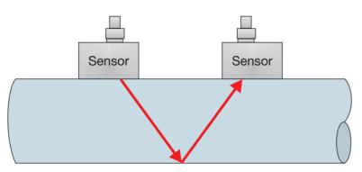
Figure 13. Clamp-On Transducer Placement
