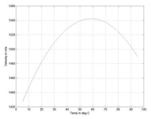
Figure 14. Ultrasound Velocity in Water as a Function of Water Temperature
