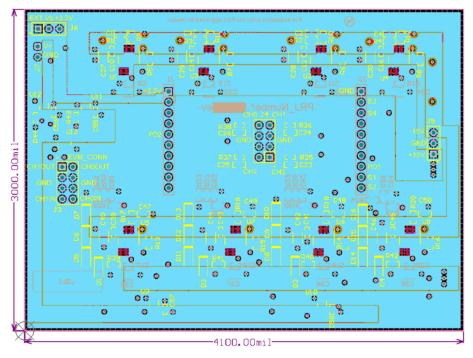
Figure 24. GND Fill on Layer Two
