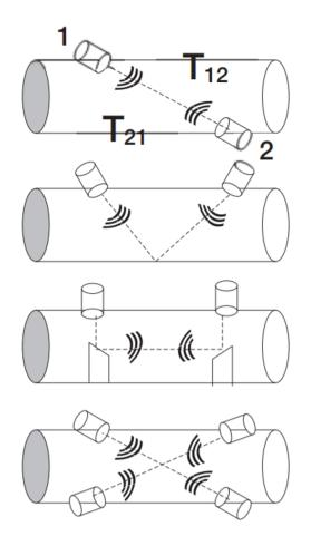
Figure 12. Various Configurations of In-Line Placement of Transducer Pairs
