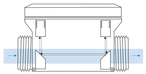
Figure 11. In-Line and Reflective Transducer Placement
