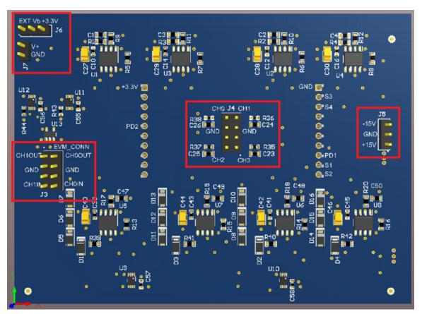
Figure 19. TIDA-01486 Hardware Configuration
