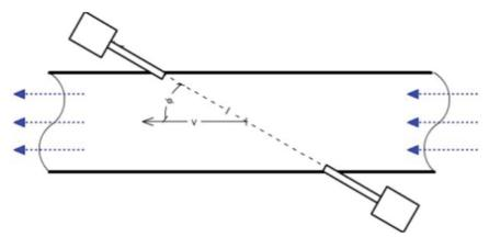
Figure 10. In-Line and Diagonal Transducer Placement
