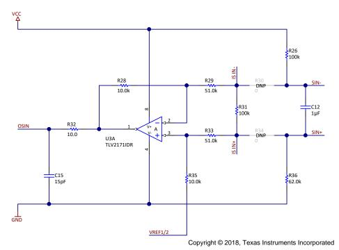
Figure 13. Resolver Feedback Winding Monitoring
