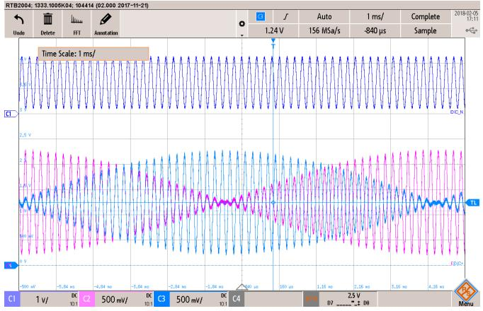
CH1 – Exciter voltage monitoring (OEXC); CH2 – Sine-winding voltage monitoring (OSIN); CH3 – Cosine-winding voltage monitoring (OCOS)
