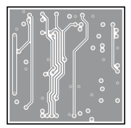
Figure 37. Internal Layer 2 With Power Rail VCC and Signals
