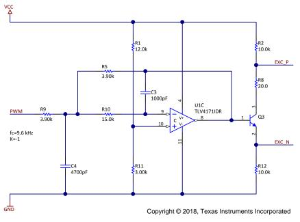
Figure 6. Multiple-Feedback Filter (MFB) in TIDA-01527
