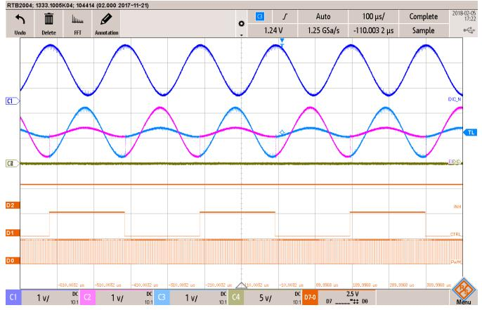
D0 – Input PWM from the C2000 MCU; D1, D2 - Control (CTRL) and Inhibit (INH) signals for the analog crossbar; CH1 – Exciter voltage monitoring (OEXC), CH2 – Sine-winding voltage monitoring (OSIN); CH3 – Cosine-winding voltage monitoring (OCOS).
