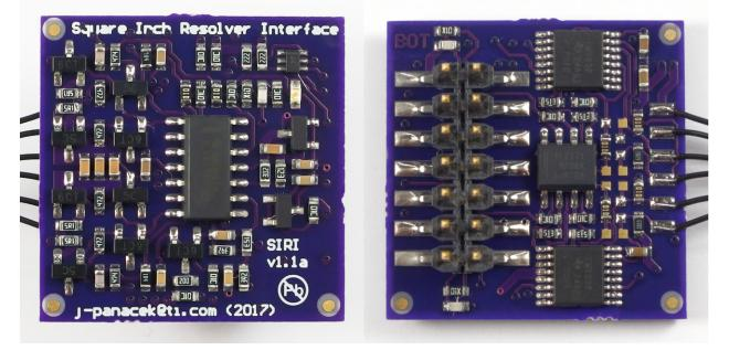
Figure 1. TIDA-01527 Board (Top and Bottom)
