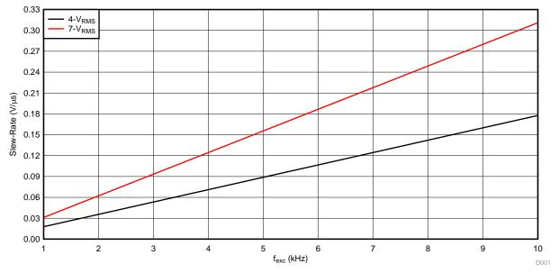
Figure 8. Minimum Required Slew Rate per Amplifier (Single-Ended) for 4-V<sub>RMS</sub> and 7-V<sub>RMS</sub> Resolvers
