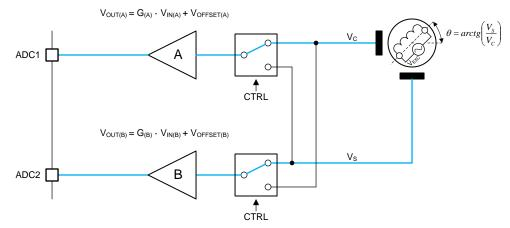
Figure 18. Scattered Signal Processing Method—Step 2: Direct Mode
