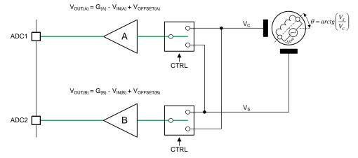
Figure 17. Scattered Signal Processing Method—Step 1:DC Offset Calibration
