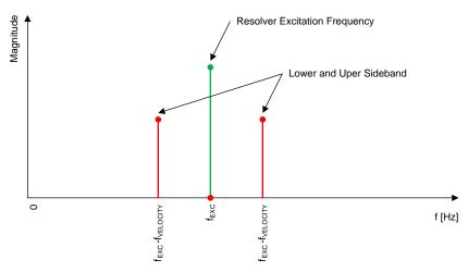
Figure 10. Magnitude Spectrum of Resolver Sensor Output Signal
