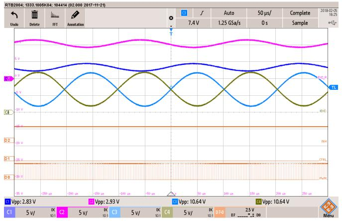
D0 – Input PWM from the C2000 MCU; D1, D2 – Control (CTRL) and Inhibit (INH) signals for the analog crossbar; CH1, CH2 – Generated sine wave after the analog phase-splitter (EXC\_N, EXC\_P); CH3, Ch4 – Excitation amplifier outputs (EXC+, EXC–)
