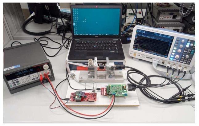
Figure 22. TIDA-01527 Test Setup Used for Development and Measurements
