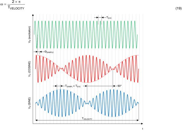
Figure 14. Typical Resolver Waveforms
