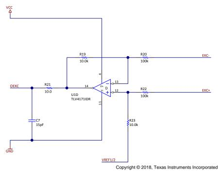
Figure 12. Excitation Amplifier Output Monitoring
