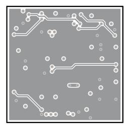
Figure 36. Internal Layer 1 With Common Ground GND and Signals
