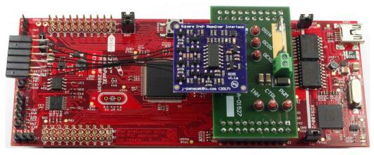
Figure 21. LAUNCHXL-F28069M Development Board With TIDA-01527 and LaunchPad™ Adapter
