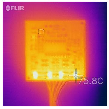
Figure 33. TIDA-01527 Thermal Imaging Camera Picture
