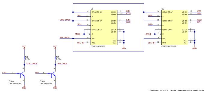
Figure 11. Analog Crossbar (Experimental)
