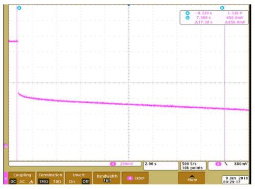
Figure 16. Discharge of Capacitive Load Without Fast Discharge Circuit
