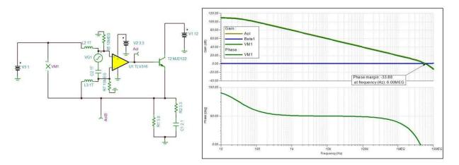
Figure 8. TINA-TI™ Stability Analysis of EC Mirror Driver Without Compensation
