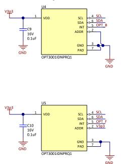
Figure 6. Ambient Light Sensors Schematic
