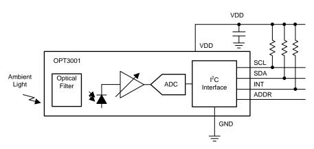
Figure 2. OPT3001-Q1 Block Diagram
