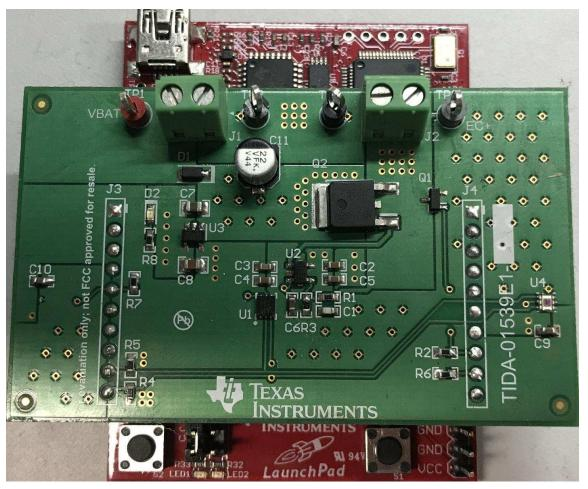
Figure 13. Image of TIDA-01539 Connected to MSP-EXP430G2552 LaunchPad™
