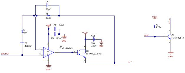
Figure 10 shows the EC mirror driver schematic.
