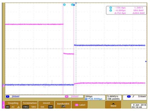
Figure 17. Discharge of Capacitive Load With Fast Discharge Enabled
