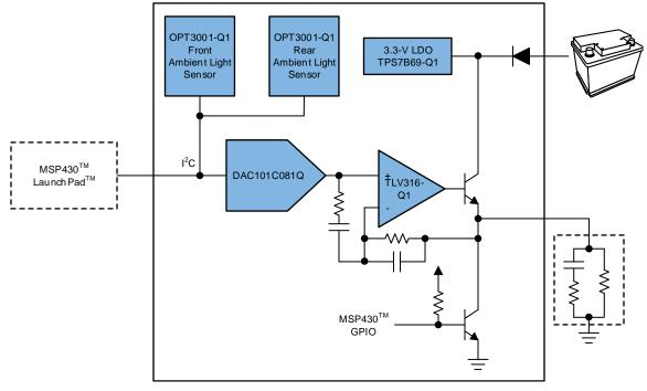
Figure 1. TIDA-01359 Block Diagram
