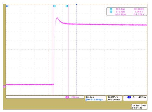
Figure 15. Impulse Response of EC Mirror Driver Stage With Typical Electrochromic Load
