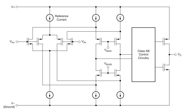
Figure 5. TLV316-Q1 Block Diagram
