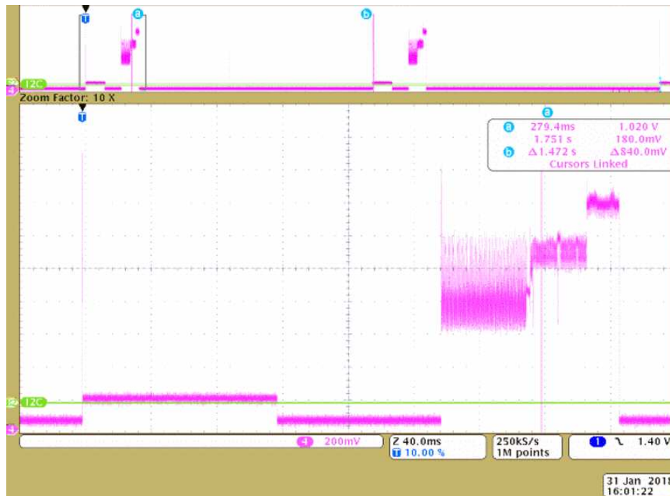
Figure 6. System Current Consumption
