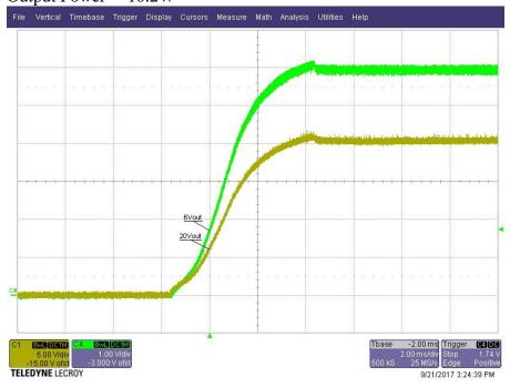
Input voltage = 230VAC Output Power = 10.2W
