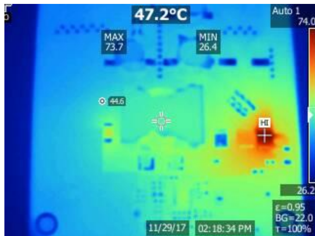
IR thermal image taken at steady state with 12Vin and 7.5A load (no airflow; ambient at room temp.)
