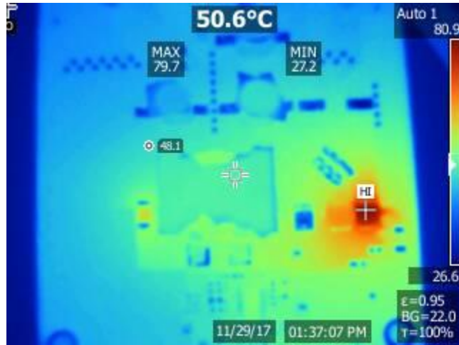
IR thermal image taken at steady state with 10.8Vin and 7.5A load (no airflow; ambient at room temp.)
