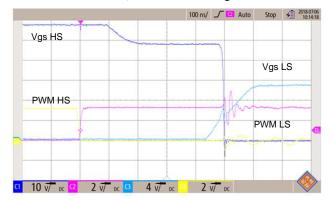
Figure 18. 6-Mode PWM vs  $V_{GS}$  LS and HS, Phase A Current at 48 V, 5 A Soft Switching
