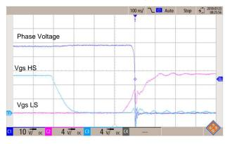
Figure 11. Soft Switching Phase A Voltage Rising Edge, Phase Current at 48 V, 10 A
