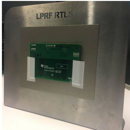
Figure 18. PCB With Metal Structure Setup - Back
