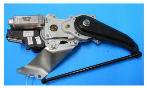
Figure 1. Liftgate Mechanism
