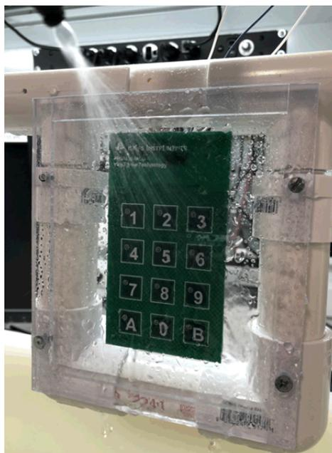
Figure 20. Continuous Water Spray Test Setup
