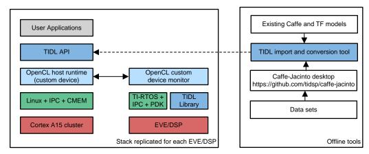
Figure 8. TIDL Software Stack
