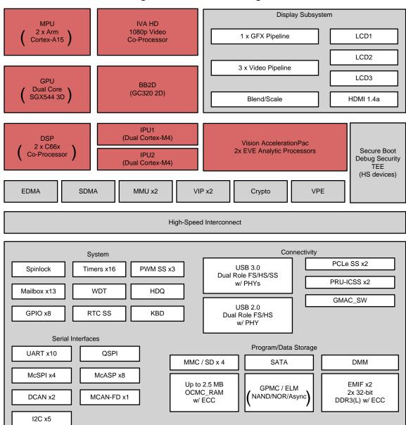
Figure 1. AM574x Block Diagram
