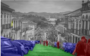
TI developed an example network model named as JacintoNet11 to demonstrate object classification, JDetNet model to demonstrate object detection and JSegNet21 to demonstrate pixel-level semantic segmentation.
