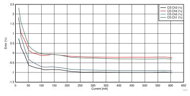
Figure 3-13. Error of Current Measurement
