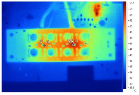
Figure 3-14. IO-Link® Master Thermal Image at 1-A Load per Port
