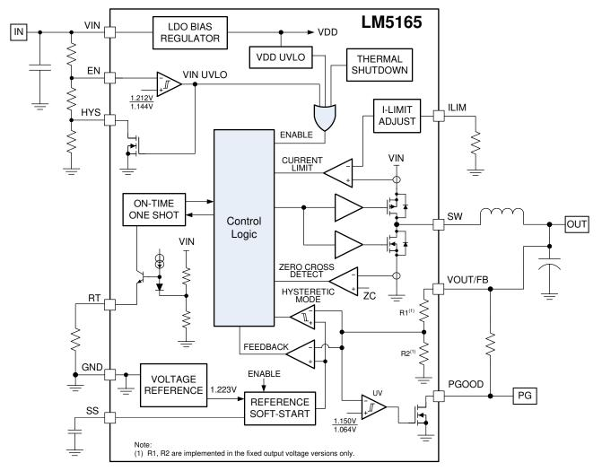
Figure 2-2. LM5165 Block Diagram
