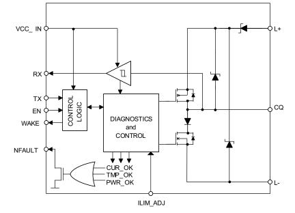
Figure 2-6. TIOL111 Block Diagram
