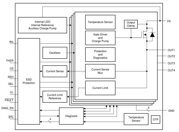
Figure 2-4. TPS4H160 Block Diagram
