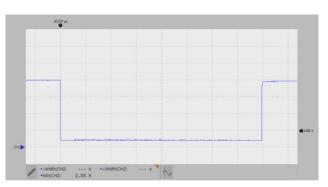
Figure 3-4. Testcase TCM\_PHYL\_INTF\_IQWUL: Low-Side Driver, Load = 24  $\Omega$ , 20-V Supply, 5 V/div, 10  $\mu$ s/div
