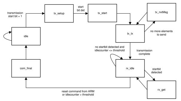
Figure 2-13. State Machine of the Frame-Handler Simplified Overview
