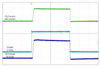
Figure 2-7. Test Results of TIOL111 Device Wake-Up Pulse
