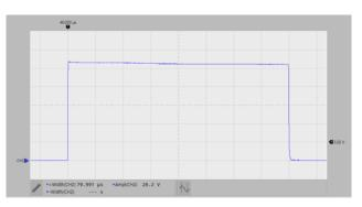
Figure 3-3. Testcase TCM\_PHYL\_INTF\_IQWUH: High-Side Driver, Load = 26  $\Omega$ , 30-V Supply, 5 V/div, 10  $\mu$ s/div
