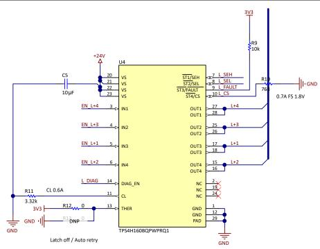
Figure 2-10. High-Side Switch Schematic
