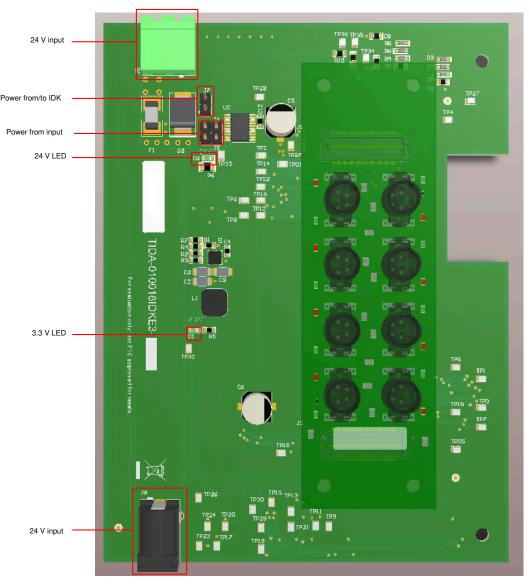
Figure 3-1. Power Connectors and Jumpers
