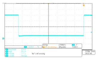
Figure 3-10. Testcase TCM\_PHYL\_INTF\_IQPKLM: Wake-Up Current Low Side - 20 V L+ Resulting in 2 V
