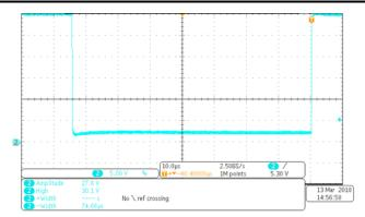
Figure 3-11. Testcase TCM\_PHYL\_INTF\_IQPKLM: Wake-Up Current Low Side - 30 V L+ Resulting in 2 V
