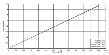
Figure 3-12. Output Voltage of TPS4H160 vs Current
