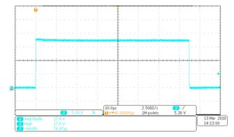
Figure 3-8. Testcase TCM\_PHYL\_INTF\_IQPKHM: Wake-Up Current High Side - 20 V L+ Resulting in 17.4 V
