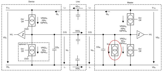
Figure 2-8. Block Diagram IO-Link® System
