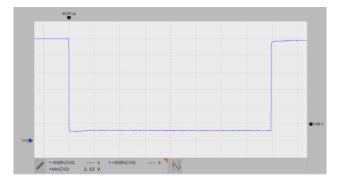
Figure 3-5. Testcase TCM\_PHYL\_INTF\_IQWUL: Low-Side Driver, Load = 44  $\Omega$ , 30-V Supply, 5 V/div, 10  $\mu$ s/div
