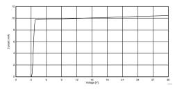
Figure 3-7. Input Current on the CQ Line
