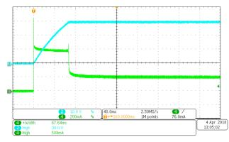
Figure 3-6. Testcase TCM\_PHYL\_INTF\_ISIRM: – Power-On Supply Current Capability
