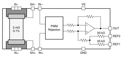
Figure 2-5. INA253 Block Diagram
