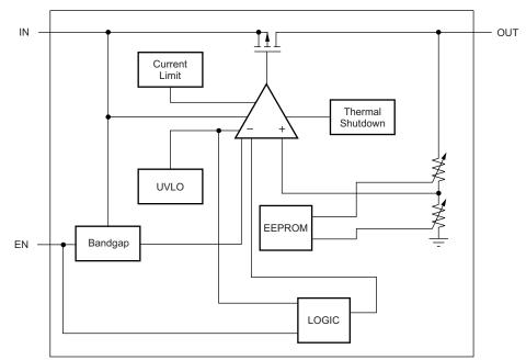
Figure 4. TPS727 Functional Block Diagram
