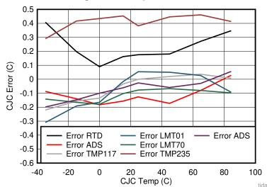
Figure 37. Temp Error CJC
