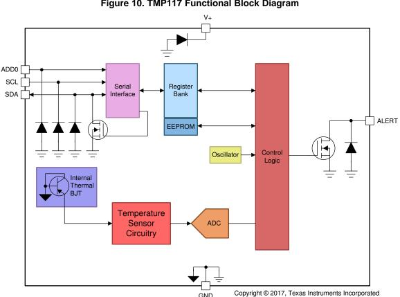
Figure 10. TMP117 Functional Block Diagram
