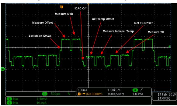
Figure 43. Current Profile RTD with Offset Compensation
