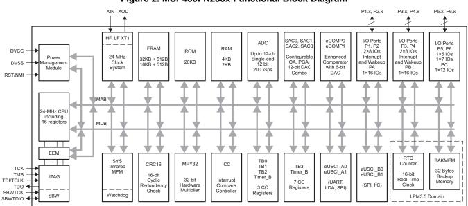
Figure 2. MSP430FR235x Functional Block Diagram
