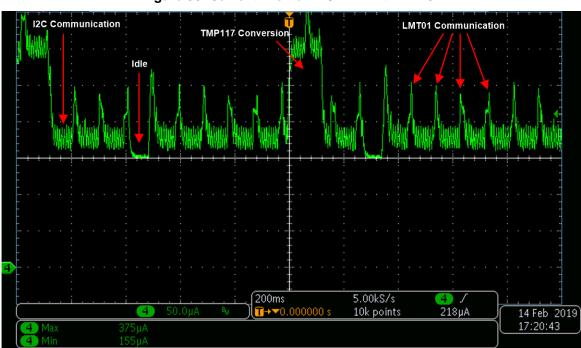
Figure 50. Current Profile ADS7142 with LMT01
