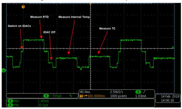
Figure 42. Current Profile RTD no Offset Compensation
