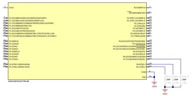
As shown in Figure 30, all interfaces to the sensors and ADCs are brought out to a standard 2.54-mm header for debug and development access. This can either be used to monitor and debug the communication, or to attach an external microcontroller without modification of the board.
