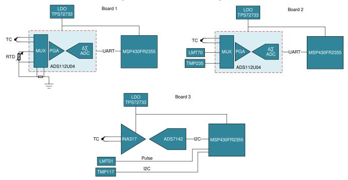
Figure 1. TIDA-010019 Block Diagram
