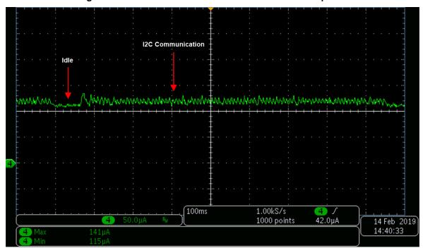
Figure 48. Current Profile ADS7142 Reference and Amplifier
