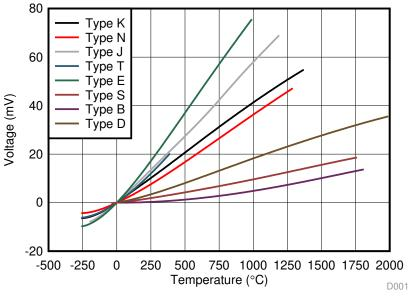
Figure 16. Overview Thermocouples
