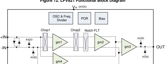
Figure 12. LPV821 Functional Block Diagram
