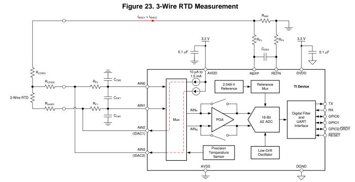
To measure the RTD, the MUX and the PGA must be configured as shown in the Table 3. This enables the current sources, set to 250  $\mu$ A each, and routes them to the RTD and the reference resistor. The voltage drop over the reference resistor is selected as a reference for the ADC. This gives a ratio metric measurement for the RTD in a 3-wire configuration, canceling out the wire resistance.
