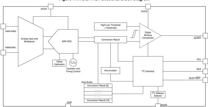
Figure 14. ADS7142 Functional Block Diagram
