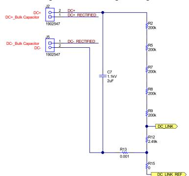
Figure 5. DC Link Voltage Sensing
