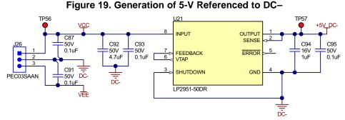
The control card requires a 3.3-V rail and a 5-V rail which are referenced to primary side ground. The 3.3-V rail is used to power the LaunchPad, analog signal conditioning circuit and the comparator circuit on the control card. The 5-V rail is used to power the PWM drive buffer and sent from the control card to the inverter power board where it is used to power the primary side of the isolated amplifiers.
