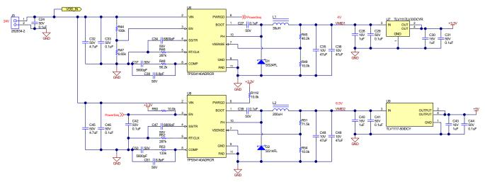
Figure 20. Low-Voltage Side DC Power-Supply Rails Generation
