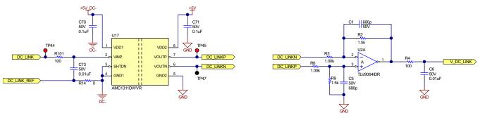
Figure 6. DC Bus Voltage Sensing Using AMC1311
