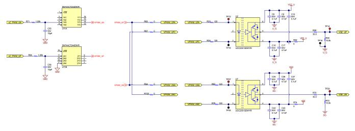
Figure 9. Buffer Used to Interlock High-Side and Low-Side Gate Drivers
