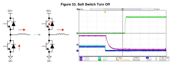
Figure 34 and Figure 35 show the turn on and turn off dv/dt of the inverter switch node captured at 2-A phase current at a DC link voltage of 565 V. Note that the turn off dv/dt depends on the phase current and the output capacitance Coss of the IGBT. Higher the phase current faster the voltage builds up across the Coss.
