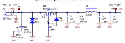
Figure 3. Input Filter Schematic
