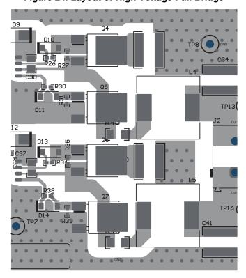
Figure 24. Layout of High Voltage Full Bridge
