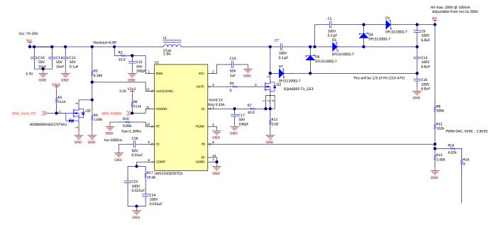
Figure 4. LM5155-Q1 Boost Schematic
