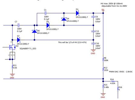
Figure 5. Voltage Tripler Schematic
