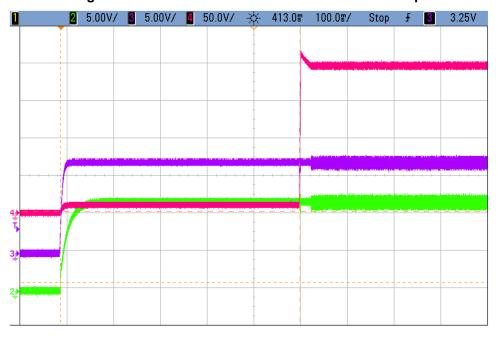
Figure 19. LM5155-Q1 and TPS61041-Q1 Boost Startup
