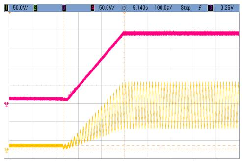
Figure 20. Ramp Up of Output Sinusoid
