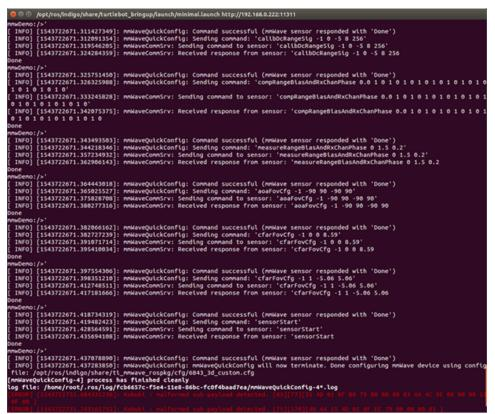
After the Kobuki and the mmWave sensor are configured, you might see this periodic "Kobuki : malformed subpayload detected" error message. These error messages come from the Kobuki driver and do not affect the operation of the demo.
