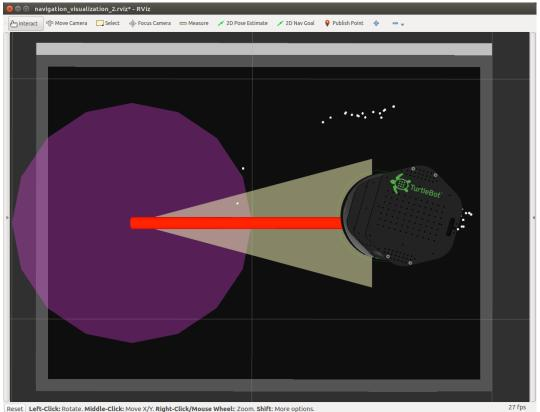
Figure 17. Ubuntu Rviz Screen Capture - Right-Side B Point Goal Reached
