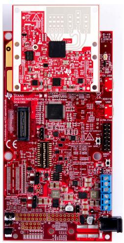
Figure 3. mmWave EVM: IWR6843ISK Mounted on MMWAVEICBOOST
