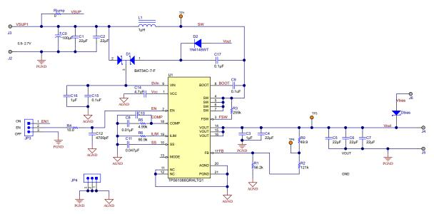
Figure 3. TPS61088 Boost Converter
