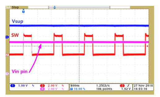
Figure 9. SW and VIN Pin Waveform When Vsup = 1.2 V
