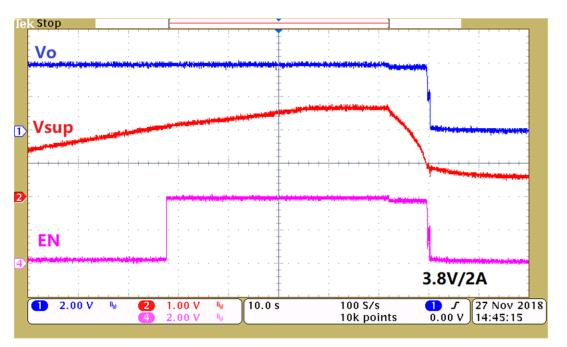
Figure 7. Working Sequence at  $V_o = 3.8 V$ ,  $I_o = 2 A$
