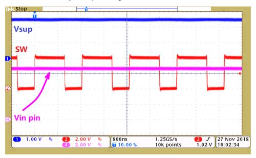
Figure 8. SW and VIN Pin Waveform When Vsup = 2.5 V
