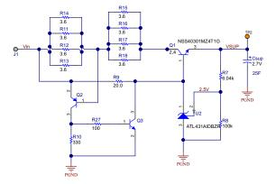
Figure 2. Super-Capacitor Charge Circuit
