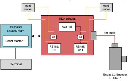
Figure 30. Block Diagram of Test Setup Used for Current Consumption
