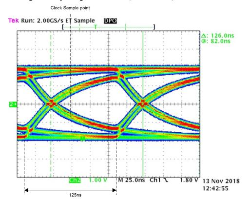
Figure 12. Eye Diagram THVD1450, 100-m Cable, 8-MHz Data Rate
