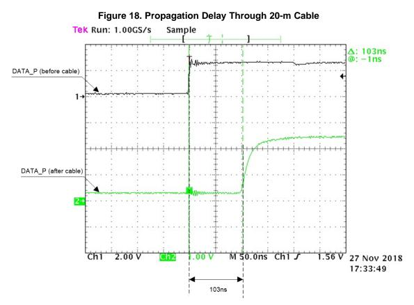
To know the cable delay through the HEIDENHAIN cable, the differential transmit signal was measured at the start and end of the cable. Table 12 and Figure 18 show the results of this measurement.
