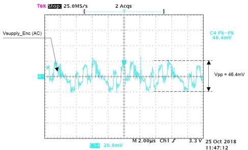
Figure 25. Encoder Voltage Output Ripple Performance With Encoder (Condition 3)
