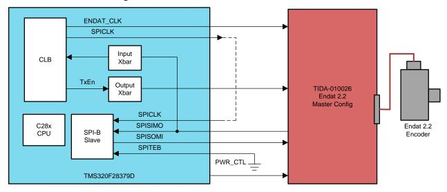
Figure 5. Endat 2.2 Master C2000 Pin Connections
