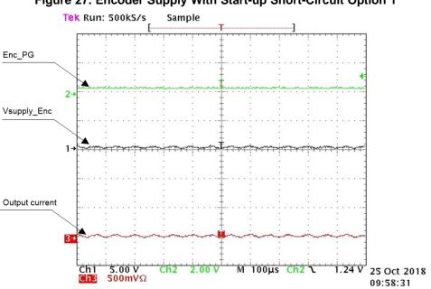
Figure 27. Encoder Supply With Start-up Short-Circuit Option 1
