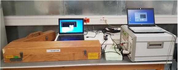
Figure 35. TIDA-010026 Test Setup for EFT Immunity Tests Using Encoder
