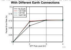
Figure 42. TIDA-010026 Test Result of the EFT at 100-kHz Test
