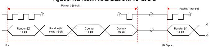
Figure 9. Test Pattern Transmitted Over RS-485 Link
