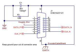
Figure 39. TIDA-010026 Schematic of Logic GND to Earth Decoupling
