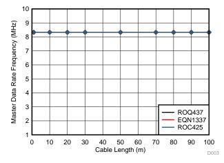
**NOTE:** The 8.33-MHz frequency of the Endat 2.2 master clock is a limit of the LaunchPad used, this can be changed to 8.00 MHz, changing the default crystal frequency of the LaunchPad.
