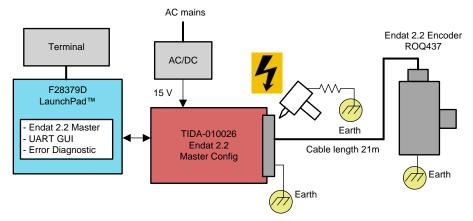
Figure 48. TIDA-010026 Test Setup for ESD Immunity Tests Using Encoder
