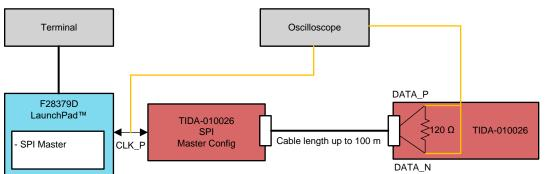
Figure 11. Block Diagram of Test Setup Used for Eye Diagram Tests
