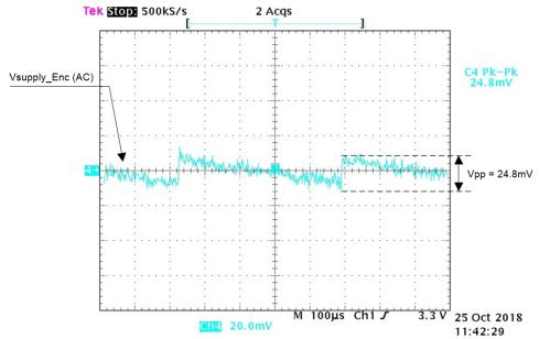
Figure 23. Encoder Voltage Output Ripple Performance With no Load (Condition 1)
