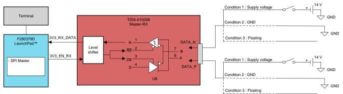
This test is conducted to test the THVD1450 device in a miss wire condition. This can happen during installation of the Encoder to the Encoder interface of the drive. For Endat 2.2 as the specification of the Encoder voltage is from 3.6 V to 14 V. The THVD1450 device is tested with a 14-V external signal on the A and B pins. After the voltage is applied to the pin, the Endat 2.2 protocol is tested on the TIDA-010026, if it is working.
