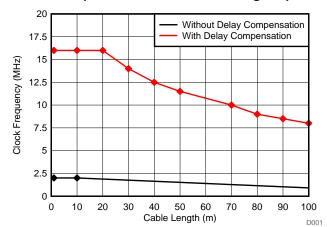
Figure 2. Maximum Clock Frequencies Versus Cable Length up to 100 m for EnDat 2.2
