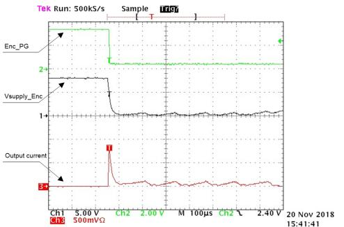
Figure 28. Encoder Supply With a Sudden Short-Circuit Option 2
