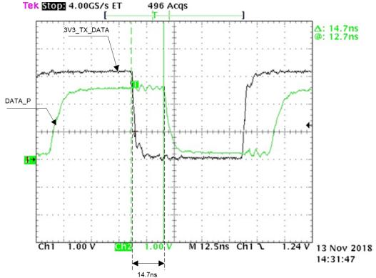
The propagation delay of the THVD1450 is within the specification of the device. The maximum delay of the driver, transmitter is 20 ns.
