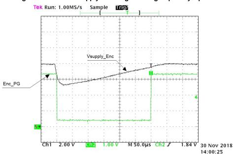
Figure 29. Encoder Supply Showing Hot-Plug Capability Option 3
