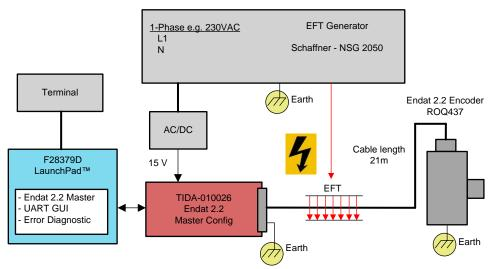
One issue of doing this test is that the encoder is a black box with an unknown RS-485 transceiver, this transceiver can influence the performance of the of the DuT. Several tests were committed with different considerations testing the RS-485 transceiver performance.
