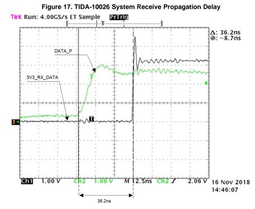
The propagation delay of the THVD1450 is within the specification of the device. The maximum delay of the receiver is 40 ns.
