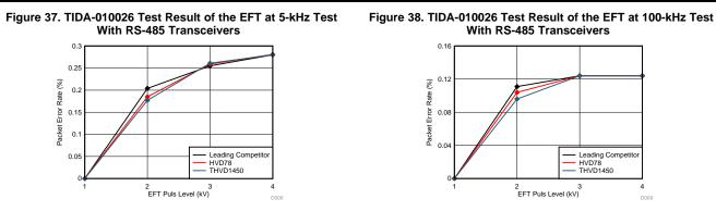
Note that the THVD1450 device performs slightly better than other high-immunity RS-485 transceivers from completion and TI at standard levels.
