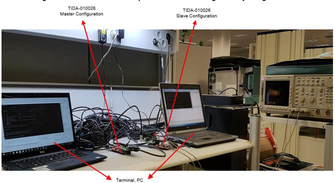
Figure 7. TIDA-010026 Test Setup for RS-485 Cable Length and Eye Diagram Tests
