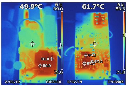
Figure 23. Thermal Image at 115-V AC, 60-Hz Input, 20-V, 5-A Output
