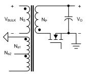
The N<sub>a1</sub> winding is designed to power the devices at 5-V and 9-V outputs. Considering the voltage derating at a light load, there should be enough margin on  $V_{DD\_min}$ . Then at a 9-V output, the  $V_{DD}$  is equal to the TVS diode voltage of 16 V. N<sub>a1</sub> must stay a small value to decrease the power consumption on the transistor.
