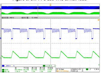
Figure 9. SW-PFC-230 VAC at Half-load
