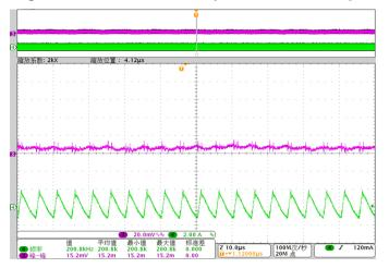
Figure 20. 115-V AC 60-HZ Input, 15-V, 5-A Output
