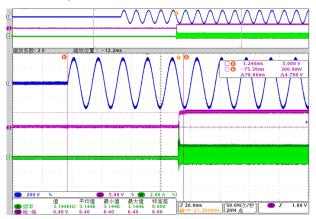
NOTE: CH1: Input Voltage; CH3: Output Voltage; CH4: Transformer Primary Current
