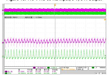
Figure 18. 115-V AC 60-HZ Input, 9-V, 5-A Output
