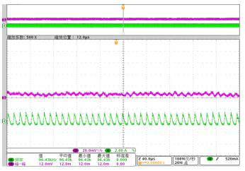
Figure 16. 115-V AC, 60-Hz Input, 5-V, 5-A Output
