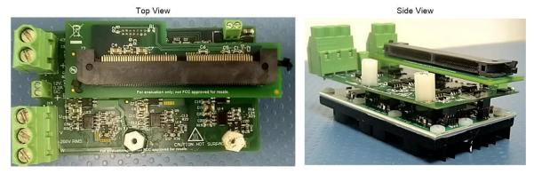
The C2000 control card can be slotted into the HSEC8 120-pin connector on the interface PCB as in Figure 17.
