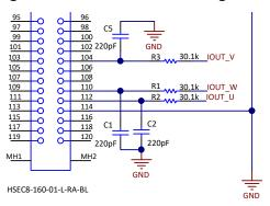
Figure 7. R-C Filter for Removing Noise
