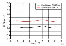
Thus, TMCS1100 enables a highly-accurate current measurement even in the presence of fast-transient switching noise. FSR is taken as 3-V for %FSR error calculation, since the reference voltage is 1.5-V.
