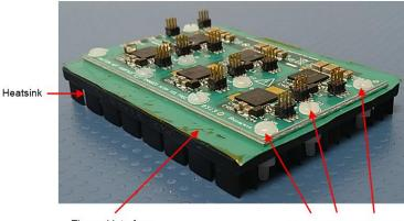
Figure 12. TIDA-010059 Power PCB Mounted on Heatsink
