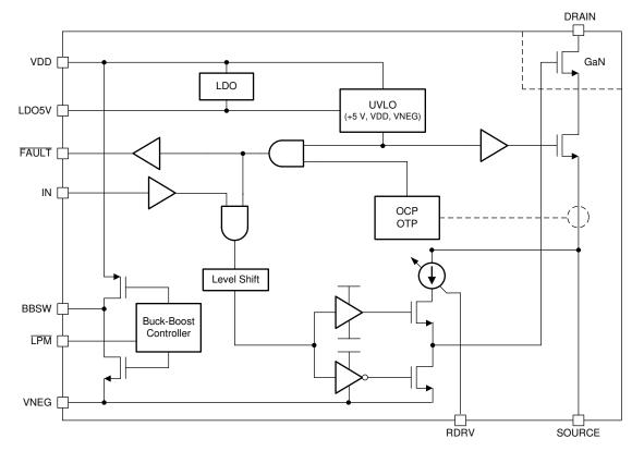
Figure 3. LMG3411R050 Functional Block Diagram
