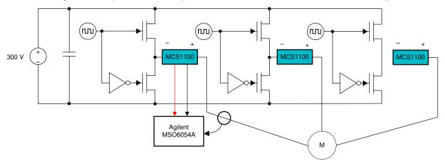
Figure 23. Experimental Setup to Estimate the Current Measurement Latency
