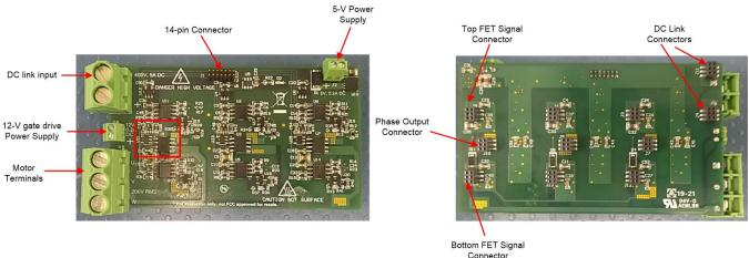
Figure 13. TIDA-010059 Current-Sensing PCB
