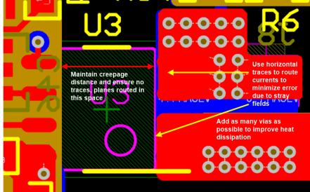
See the Layout Guidelines section of the TMCS1100 High-Precision, Isolated Current Sensor With External Reference data sheet for additional layout recommendations to enable better thermal management.
