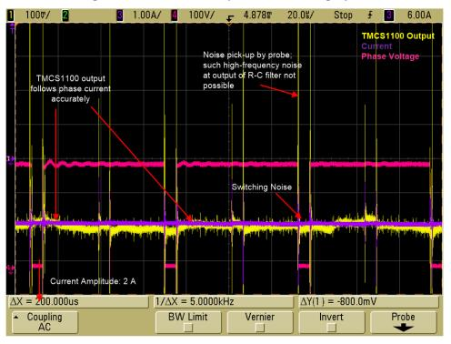
Figure 25. TMCS1100 Output in a Switching Cycle
