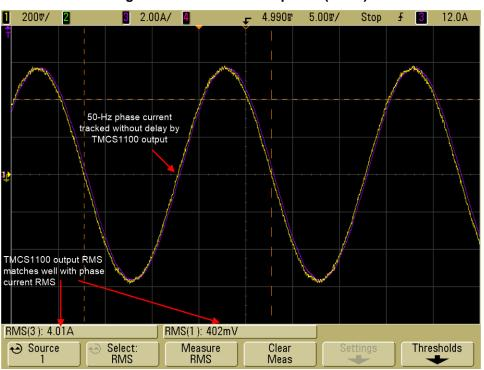
Figure 24. AC Current Response (50 Hz)
