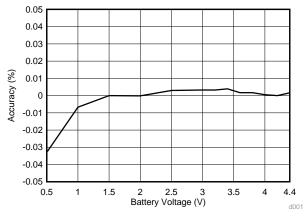
The results demonstrate that at high current levels, the ADC is able to capture current and voltage at accuracies lower than 0.01% error.
