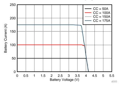
In Figure 22, with the increase in current setting, the CC control starts transforming to CV control at lower voltage. The transformation remains linear throughout testing, indicating that the ability of the design to eliminate overcharging is not affected at higher currents.
