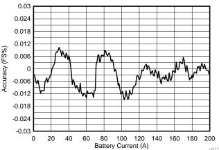
The results show that CC buck control for the entire system remains within 0.02% accuracy from 1 A to 200 A.
