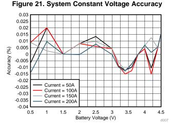
The results in Figure 21 show that the system is able to operate in CV mode with 0.01% accuracy. Table 7 lists the suggested values of calibration for voltage at different current levels of the TIDA-01042 system.
