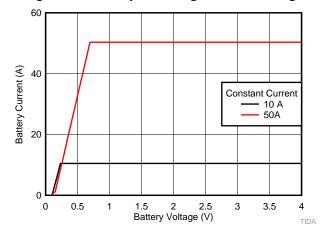
Figure 24. Battery Discharge at Low Voltage
