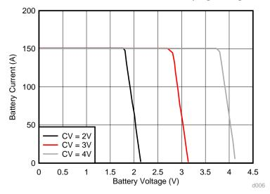
Figure 23 shows that voltage setting has less effect on the switch from CC control to CV control.
