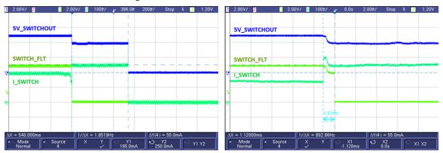
Figure 29. Encoder Current Limit at 250 mA
