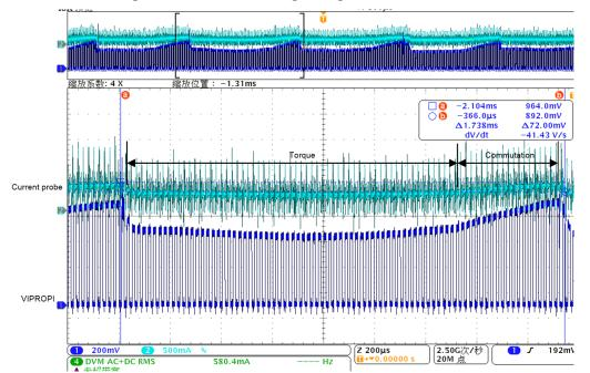
Figure 8. Current Sensing at High Load Condition
