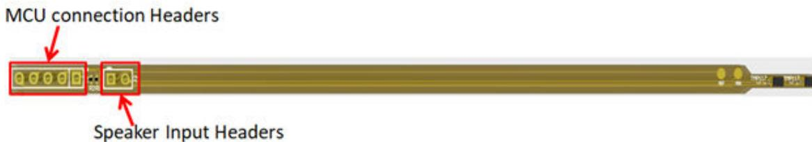
Figure 2-4. MCU and Speaker Input Headers
