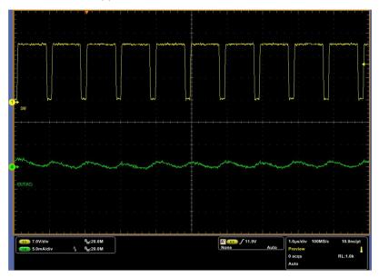
Figure 3-5. CC Mode Current Ripple
