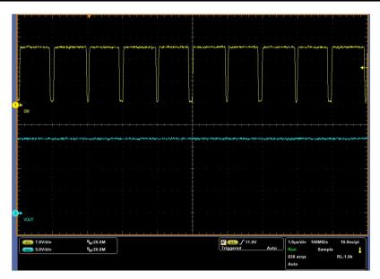
Figure 3-4. CV Mode Steady State
