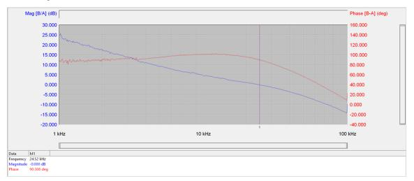
Figure 3-10. Current Open Loop Stability
