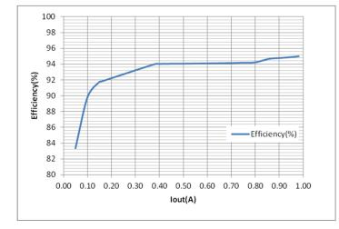
Figure 3-7 shows the efficiency curve of the battery charger across 0.1A to 1.0A.
