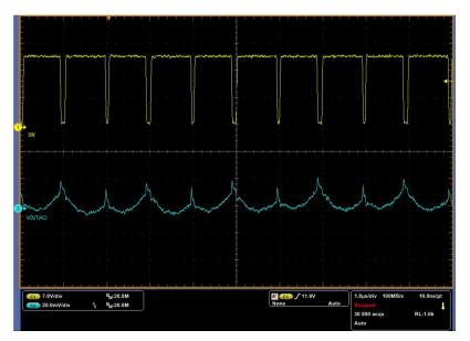
Figure 3-6. CV Mode Voltage Ripple
