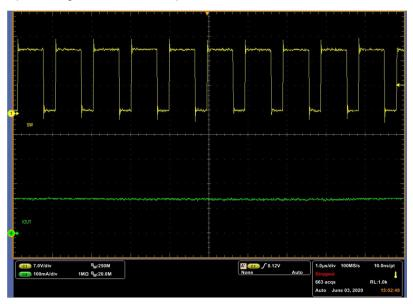
Figure 3-2. Pre-Charging Mode Steady State
