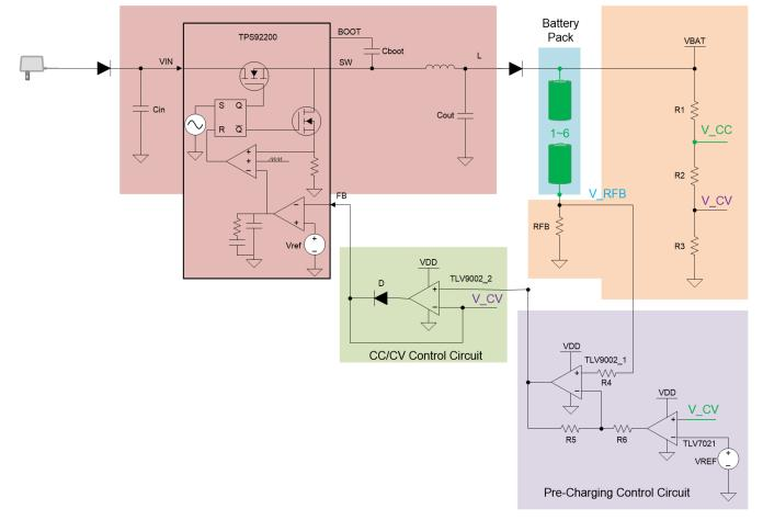
Figure 2-1. TIDA-050042 Block Diagram
