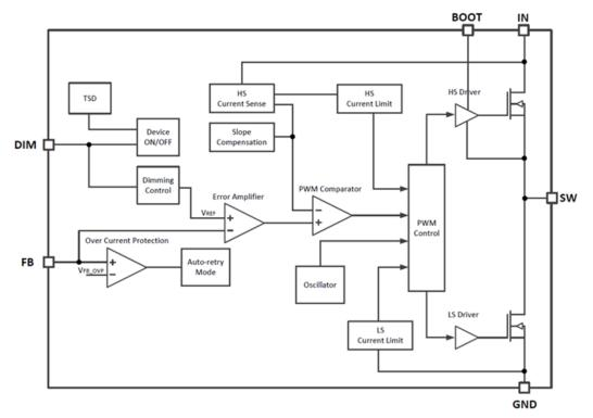
Figure 2-2. TPS92200 Functional Block Diagram
