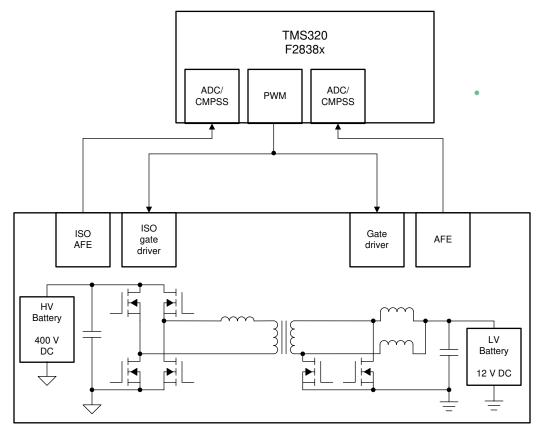
Figure 1-3. DC-DC System Block Diagram
