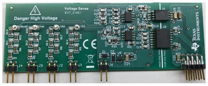
Figure 3-25. Inverter Voltage Sense Board
