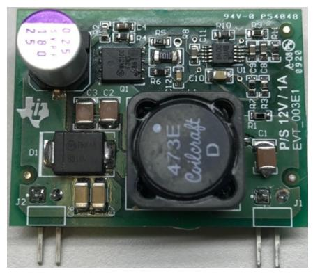
Figure 3-13. Vbat to 12-V/1-A Power Supply Module
