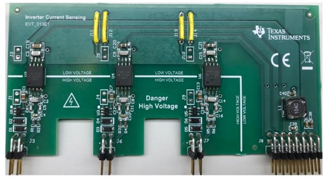
Figure 3-24. Inverter Current Sense Board
