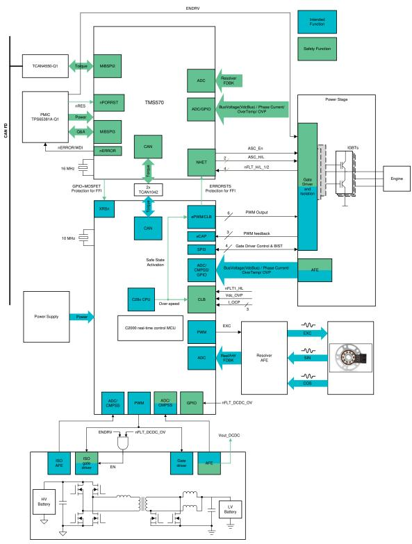
Figure 2-1. TIDM-02009 Block Diagram
