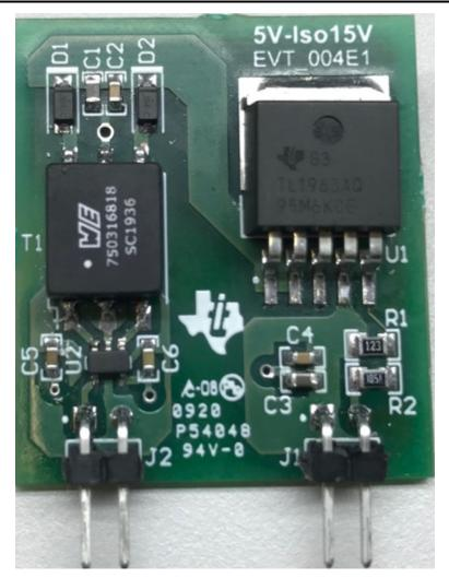
Figure 3-14. 5-V to 15-V/0.5-A power supply module
