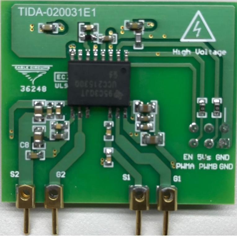
Figure 3-28. DC-DC Isolated Gate Driver
