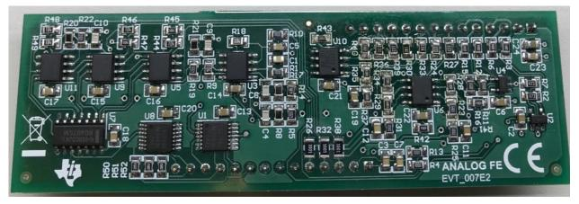
Figure 3-17. Analog Back End Module
