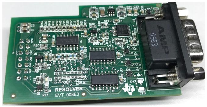
Figure 3-18. Resolver Analog Front End Module
