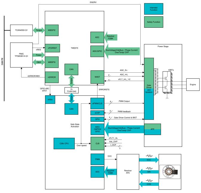
Figure 3-19. EV Traction Inverter System Block Diagram
