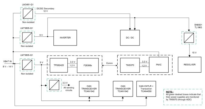
Figure 3-11. Power supply distribution
