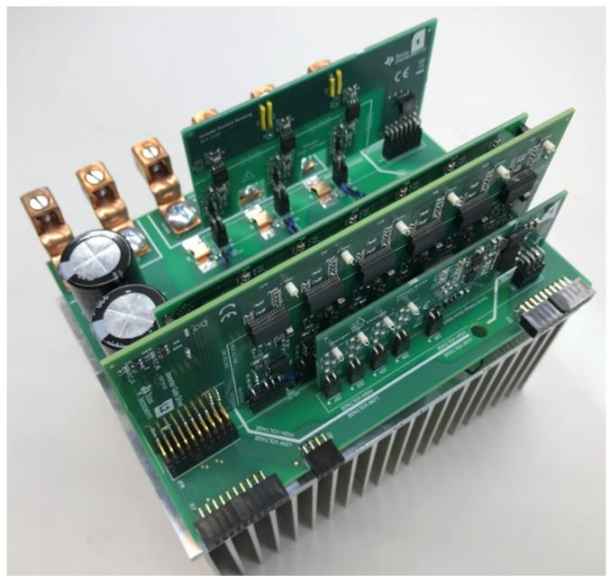
Figure 3-20. Inverter Module
