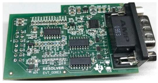
Figure 3-22. UCC5870 Gate Driver Module
