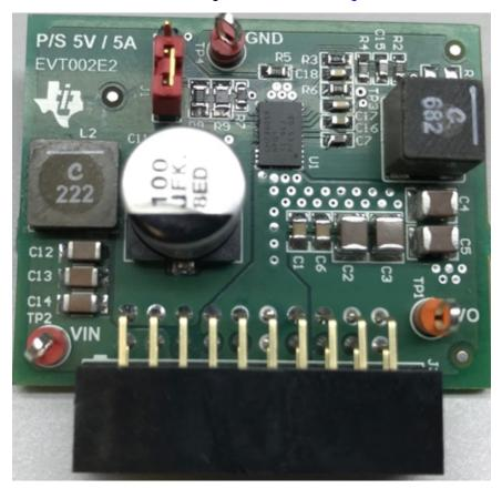
Figure 3-12. Vbat to 5V/ 5A power supply module
