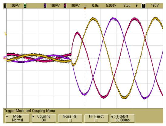
Figure 3-3. Positive-Going Transient Response (AC Load Voltage Waveforms)
