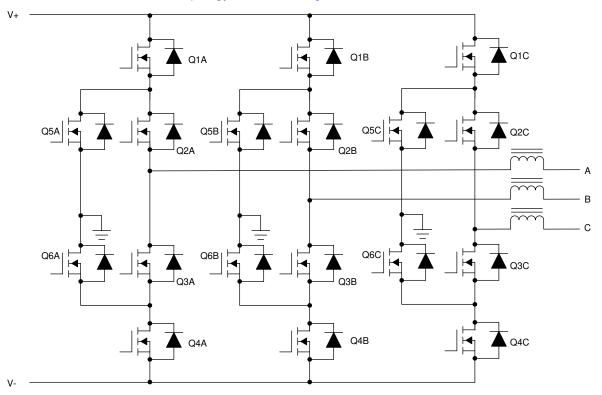
Figure 2-2. ANPC Three-Phase Inverter Architecture
