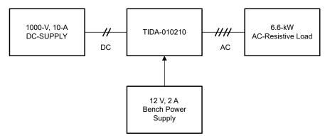
Figure 3-1. Test Setup for Resistive AC Load
