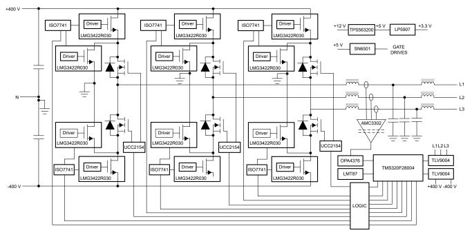
Figure 2-1. Block Diagram
