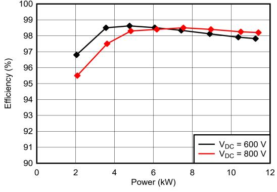
Figure 3-7. PFC Efficiency vs Input Power
