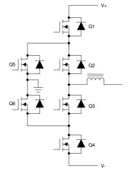
Figure 2-3. ANPC Single-Phase Inverter Leg
