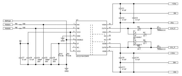
Figure 2-15. UCC21541 Gate Drive Circuit
