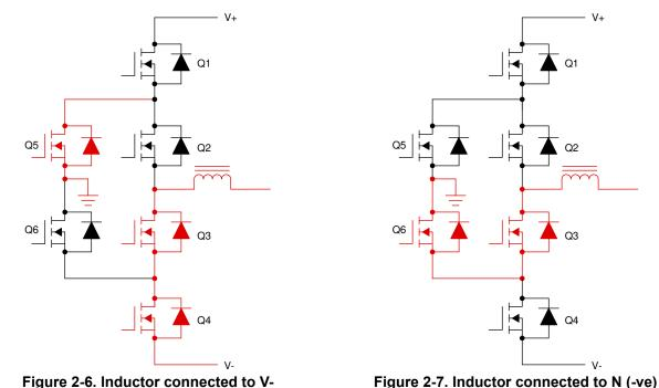
Similar to the operation during the positive half cycle, Figure 2-6 and Figure 2-7 illustrate the operation of the ANPC power stage during the negative half cycle. Q3 remains on for the entire duration of the negative half cycle.
