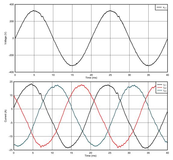
Figure 3-6. Currents and Voltage Working at 11-kVA PFC full
