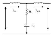
Figure 2-8. LCL Filter Architecture
