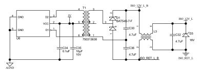
Figure 2-13. SN6501 Bias Voltage Supply for GaN Power Board
