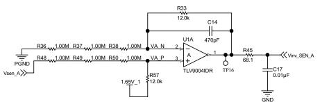
Figure 2-10. High-Voltage Sensing Signal Path
