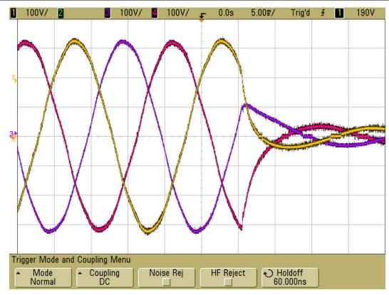
Figure 3-4. Negative-Going Transient Response (AC Load Voltage Waveforms)
