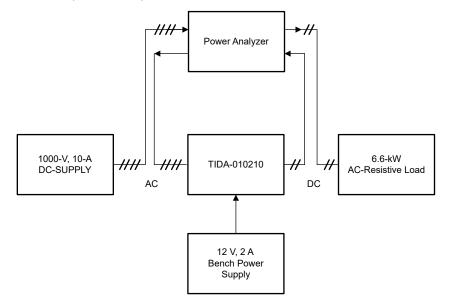
Figure 3-5. Test Setup for PFC Operation
