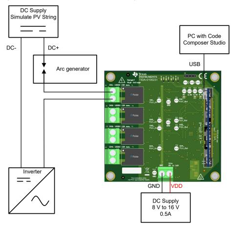
Figure 3-2. Arc Detection Test Setup
