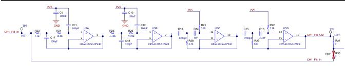
Figure 2-3. Schematic Filter Stage
