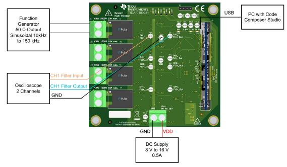
Figure 3-1. Hardware and Software Validation Setup
