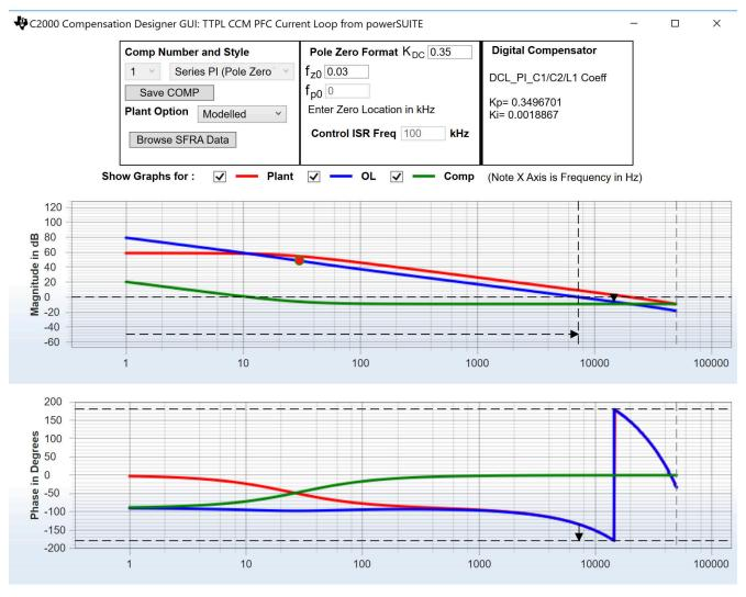
Stable Loop Folg\_cf 7.2556 kHz Gain Margin 6.21 dB Phase Margin 45.01 Degrees 🛛 🐺 TEXAS INSTRUMENTS
