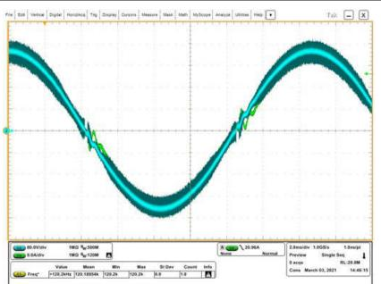
Figure 5-53. PFC Input Voltage and Input Current
