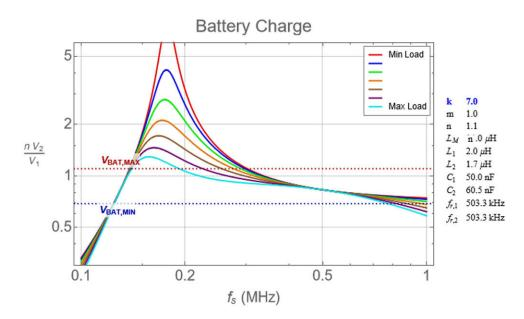
Figure 2-7. CLLLC Tank Gain Variation With L<sub>n</sub> Varying
