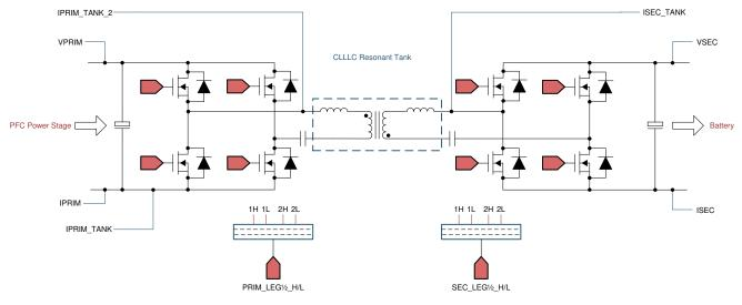
Figure 1-2. CLLLC Topology for Isolated DC-DC Converter
