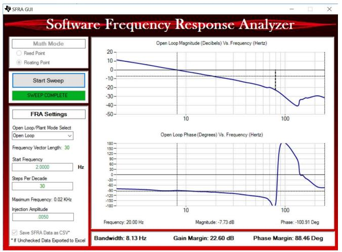
Figure 5-44. SFRA Run on Closed Voltage Loop
