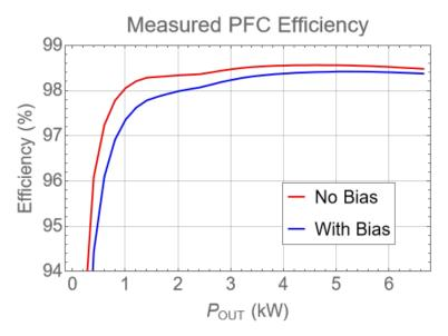
Figure 5-45. PFC Efficiency
