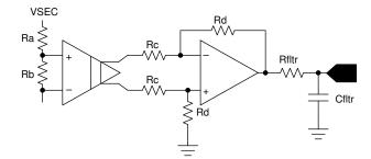
Figure 2-9. VSEC Voltage Sensing Circuit
