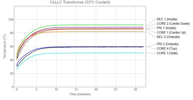
Figure 5-52. CLLLC Transformer Temperatures
