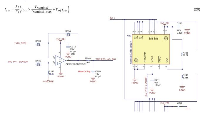
Figure 3-10. Schematic of Current Sensing
