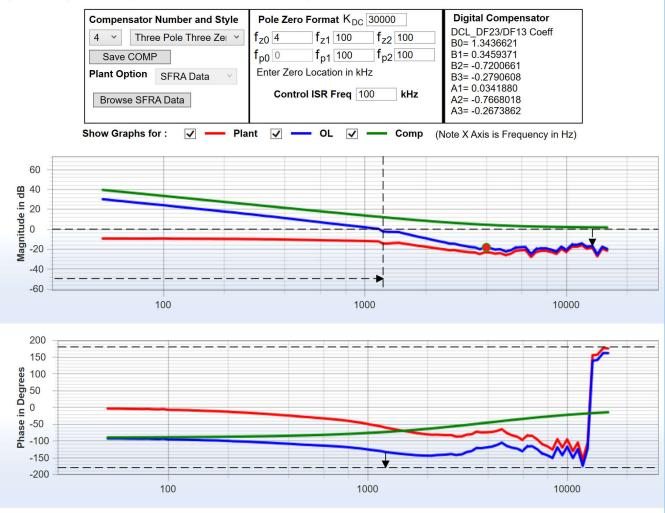
Stable Loop Folg\_cf 1.2325 kHz Gain Margin 16.78 dB Phase Margin 47.07 Degrees 🛛 🚜 Texas Instruments
