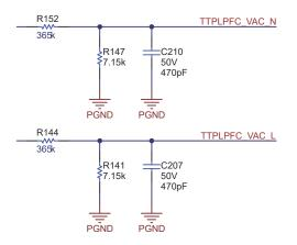
Figure 3-11. Schematic of Voltage Dividers for AC Input Voltage Sense
