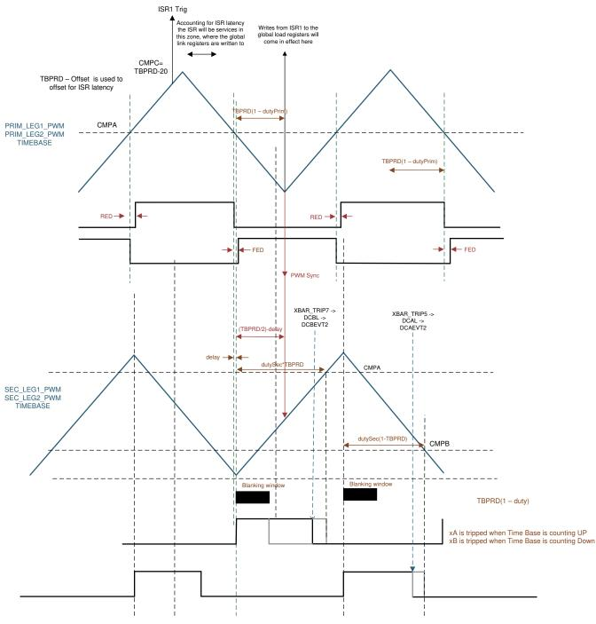
Figure 2-14. PWM Scheme Used on CLLLC Design With Active Synchronous Rectification with Power Flow Primary to Secondary
