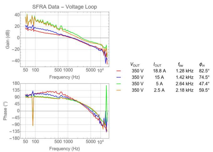
Figure 5-49. Voltage Loop Bode Plot
