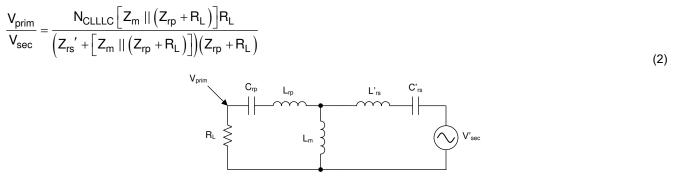
Figure 2-6. FHA Model for Gain Calculation in RCM
