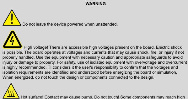
Let surface! Contact may cause burns. Do not touch! Some components may reach high temperatures > 55°C when the board is powered on. The user must not touch the board at any point during operation or immediately after operating, as high temperatures may be present.
