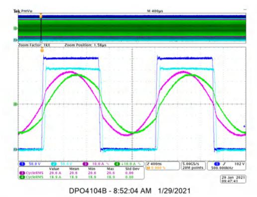
Figure 5-56. CLLLC Operation 19 A (6.6 kW)
