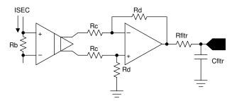
Figure 2-10. ISEC Current Sensing Circuit
