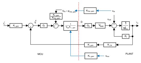
Figure 3-6. Current Loop Control Model
