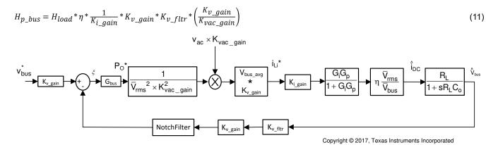
Figure 3-7. DC Voltage Loop Control Model
