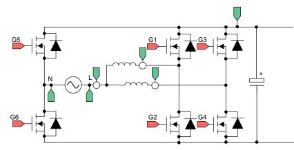
Figure 3-4. TIDM-02013 PFC Block Diagram
