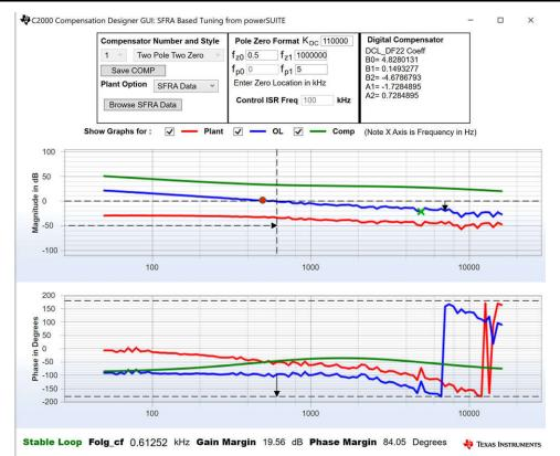
Figure 5-20. Compensator Design With SFRA Based Plant Measurement for the Voltage Loop When Resistive Load is Connected at the Output, With Measurement Data at 500kHz
