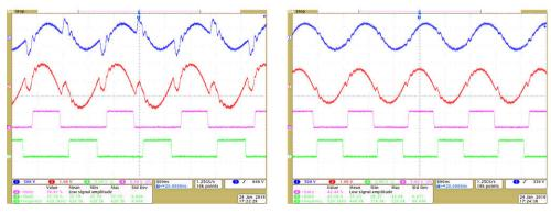
Figure 5-17. Active Synchronous Rectification Check, ch1  $\rightarrow$  IPRIM\_TANK, ch2  $\rightarrow$  ISEC\_TANK, ch3/ch4  $\rightarrow$  SEC\_LEG1\_PWMH/L
