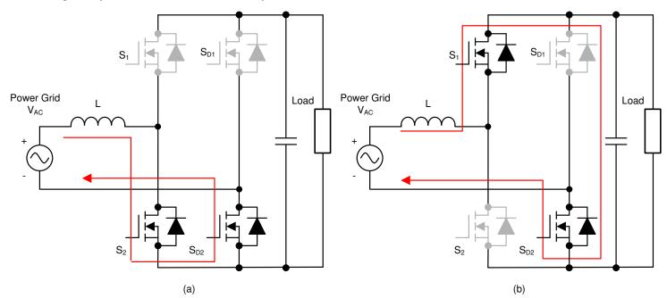
Figure 3-2. Totem-Pole Bridgeless PFC Operation During Positive Half Cycle: (A) While S<sub>2</sub> is Switched ON (B) While S<sub>2</sub> is Switched OFF
