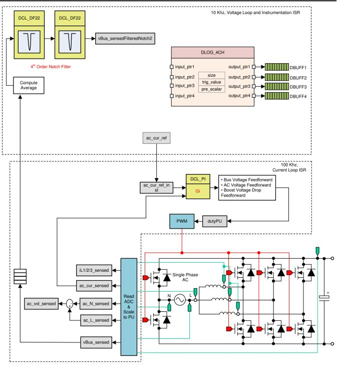
Figure 5-32. Build Level 2 Control Software Diagram: Closed Current Loop
