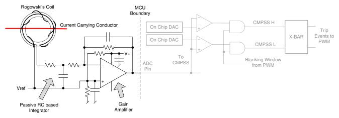
Figure 2-11. ISEC Tank Current Sensing Using Rogowski's Coil
