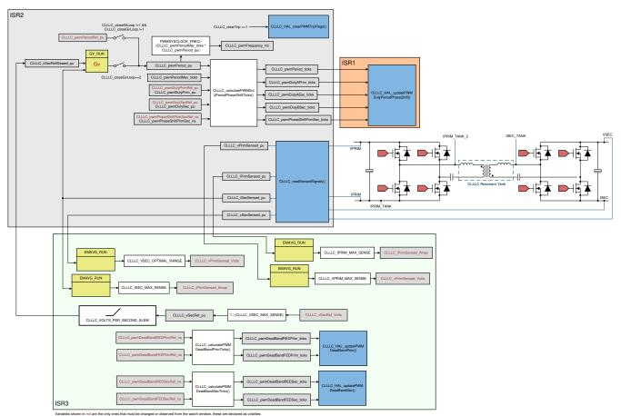
Figure 5-23. Lab 4 Control Software Diagram: Closed Current Loop
