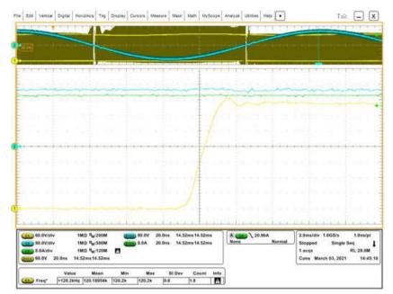
Figure 5-55. PFC GaN Drain Voltage - Transition
