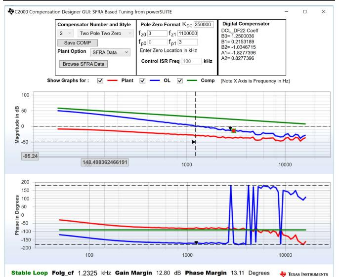
Figure 5-24. Compensator Design With SFRA Based Plant Measurement for the Current Loop, Lab 4
