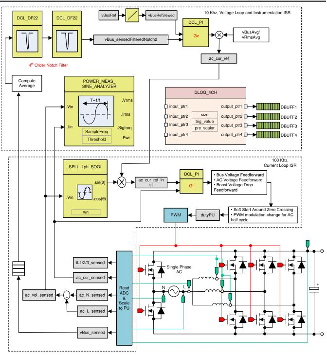
Figure 5-41. Build Level 4 Control Diagram: Output Voltage Control With Inner Current Loop
