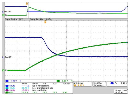
Figure 4-6. Overcurrent Protection Response Time
