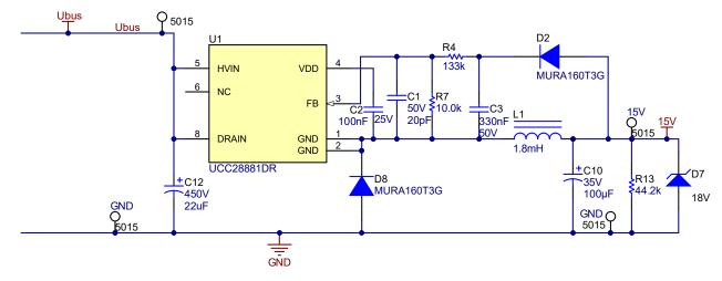
Figure 3-1. UCC28881 High-Voltage Buck Supply Circuit
