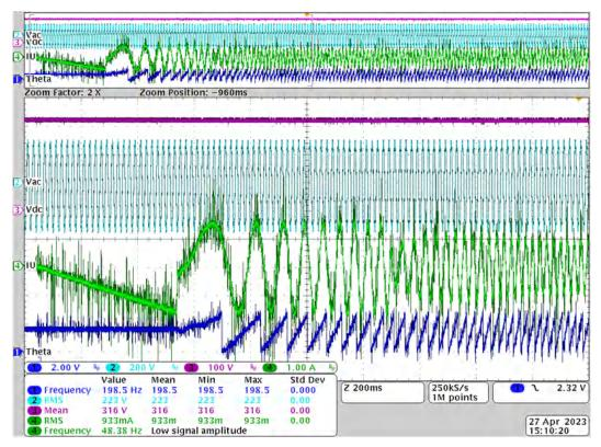
Figure 4-7. Motor Start-Up Sequence for PMSM With Senseless FOC Algorithm
