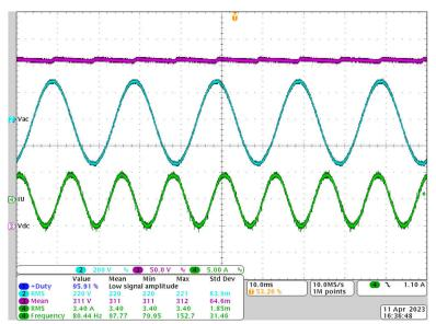
Figure 4-5. Phase Current at Open Loop Mode
