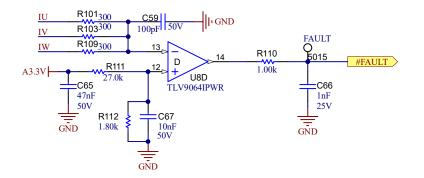
Figure 3-8. External Overcurrent Protection Circuit
