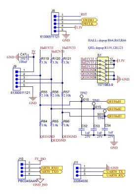
Figure 3-6. Hall and QEI Interface Circuit
