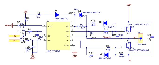
Figure 3-3. Half-Bridge IGBTs and Gate Driver
