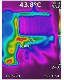
Figure 4-8. Board Temperature Rising With 460W Load
