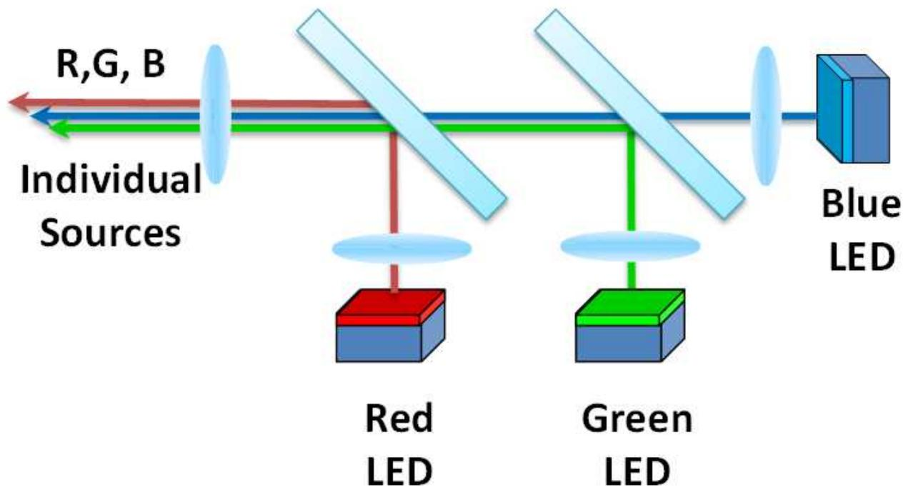
Figure 6. Typical LED Sequential Illumination
