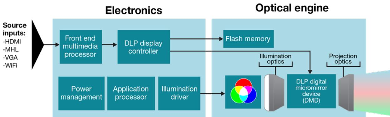
**Figure 5.** DLP Pico projection system block diagram.
