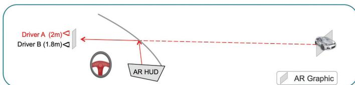
**Figure 5.** A larger eyebox supports both Driver A and Driver B
