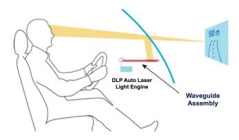
Figure 16. Waveguide based AR HUD
