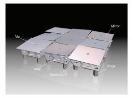
Figure 10. Example of a DMD micromirror array
