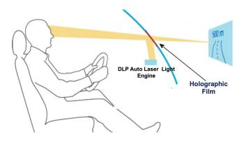
Figure 17. Holographic film based AR HUD
