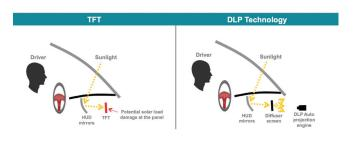
Figure 7. Comparison of a TFT-based HUD vs. a DLP technology-based HUD
