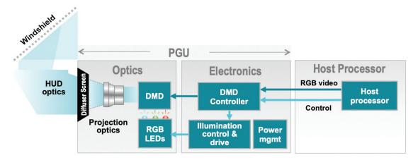
Figure 9. A DLP Auto PGU with diffuser screen
