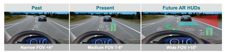
Figure 2. Future (AR) HUDs will allow for a FOV of 10 degrees or more and overlay graphics directly onto the real world
